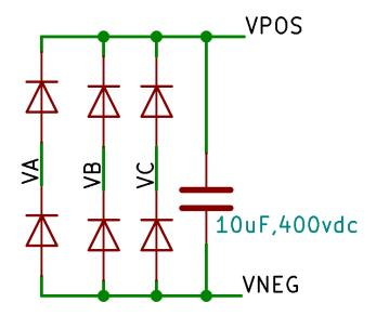
Figure 3: Drawing max 18W from AC input directly for startup & bias ring
