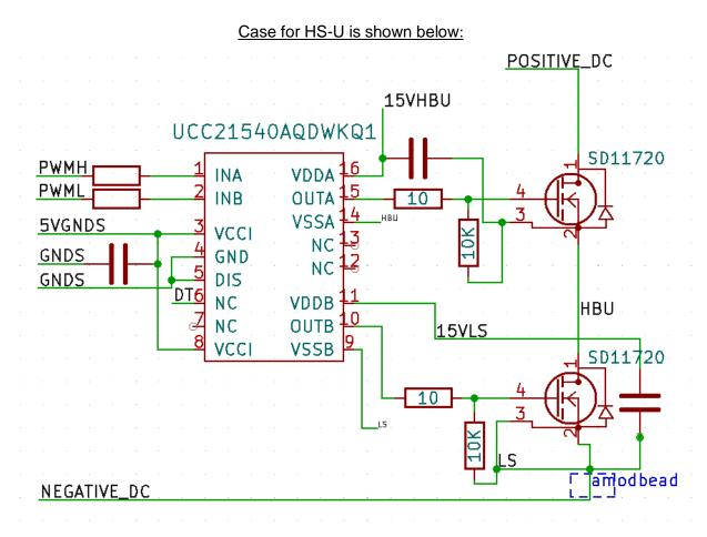
Figure 6: The totem-pole arrangement is classic Half-bridge configuration. No VEE bias option
