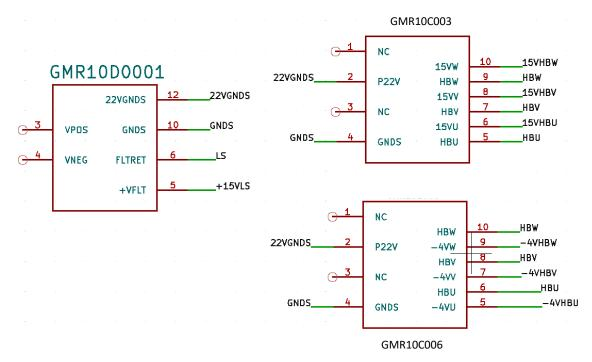
Figure 10: 3 negative bias & positive bias are independently referenced output WRT HBx
