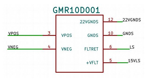
Figure 8: Ganmar Technologies GMR10D001 dual output module
