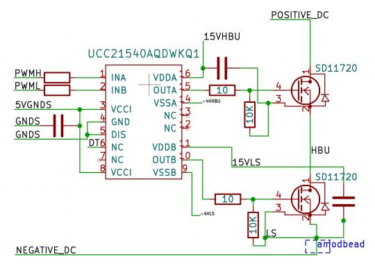
Figure 11: Half Bridge with V<sub>EEx</sub> options (HBU node shown)
