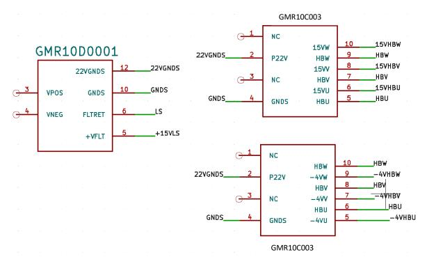
Figure 5: GMR10D001 interconnects to create HBx Power Forms using GMR10C00x
