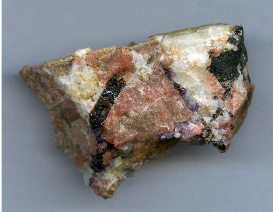
Photo 5. Fresh golden-brown euhedral prismatic crystal of fluorbritholite from the Sakhariok Massif, Kola Peninsula, Northern Region, Russia that occurs in hydrothermally altered rock. Associated minerals include pink nepheline (var. eleolite), white calcite, violet fluorite and dark green black aegirine see http://www.mindat.org/gallery.php?loc=18634
