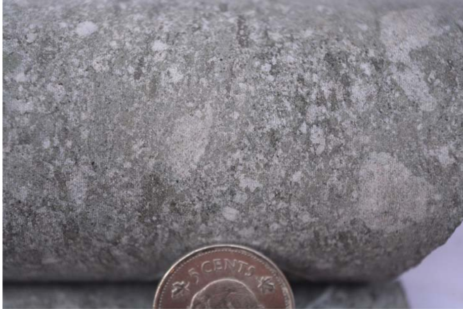
Photo 2. Ijolite breccia from 65.53 to 65.77 m drill interval showing white crystal and felsic lithic fragments.
