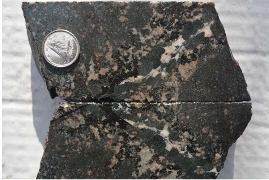
Photo 8. Mesocratic segregation at 72.2 m drill interval , which consists of coarse-grained dark-green aegirine, black phlogopite, grey nepheline and white calcite core zone, with gradation into a medium-grained ijolite host rock (upper left).
