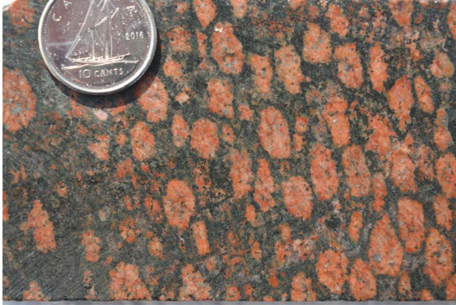
Photo 5. High concentration of orange altered nepheline megacrysts at 80 m in drill hole that reveal typical blocky to hexagonal crystal shapes.
