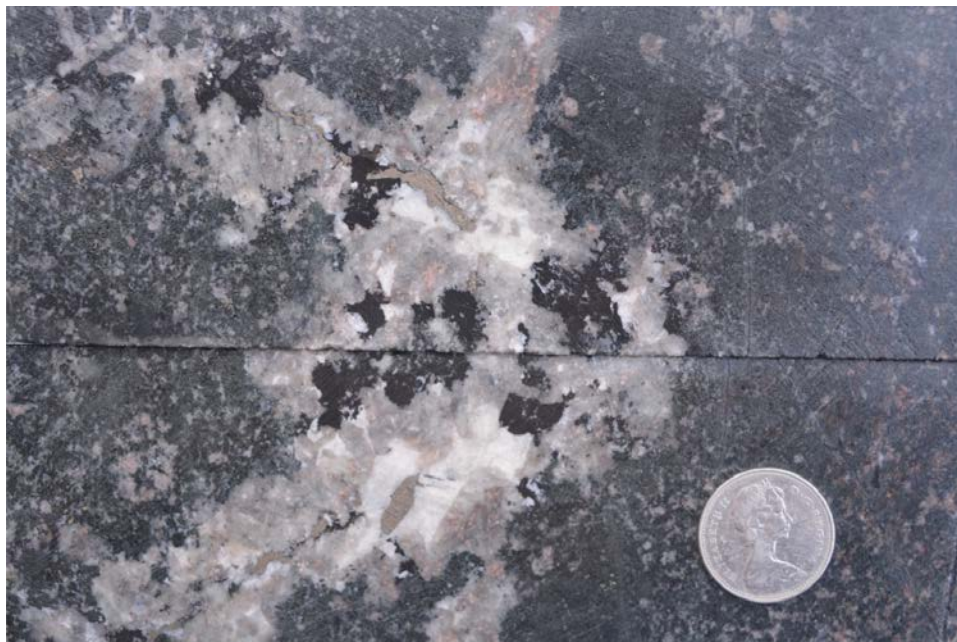
Photo 9. Leucocratic segregation of pink-grey nepheline, black phlogopite, unknown pink mineral, and white calcite in a dark green fine-to medium-grained ijolite host at 74 m drill interval. Several bronze grains of pyrrhotite occur within the segregation core area.
