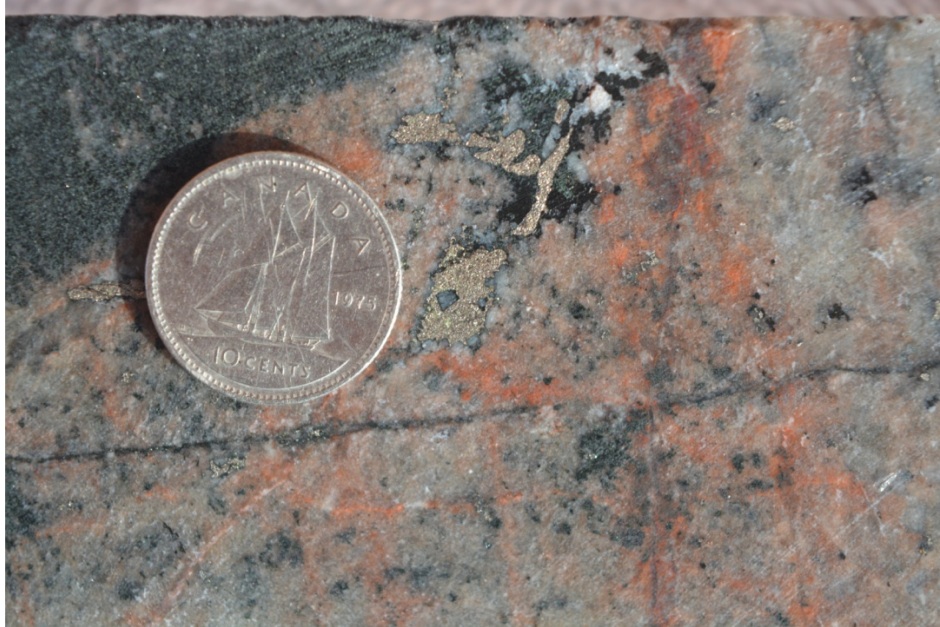
Photo 14. Light pink nepheline alteration in ijolite host near carbonatite pod at 74.47 to 74.84 m drill interval (sample 26376). Remnants of green ijolite host are exemplified in upper left corner. Note cluster of pyrrhotite associated with this type of alteration.
