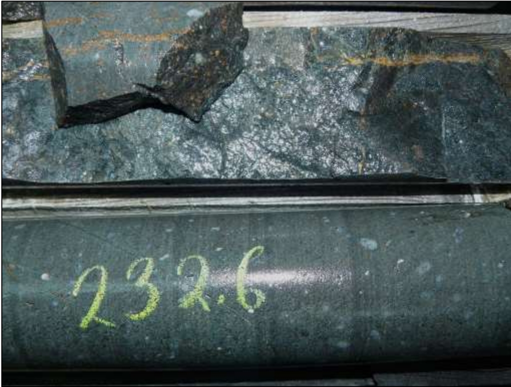
Fig. 29b. CR02-1. Litho sample at 232.6m of impure mafic rock. Note large quartz grains.
