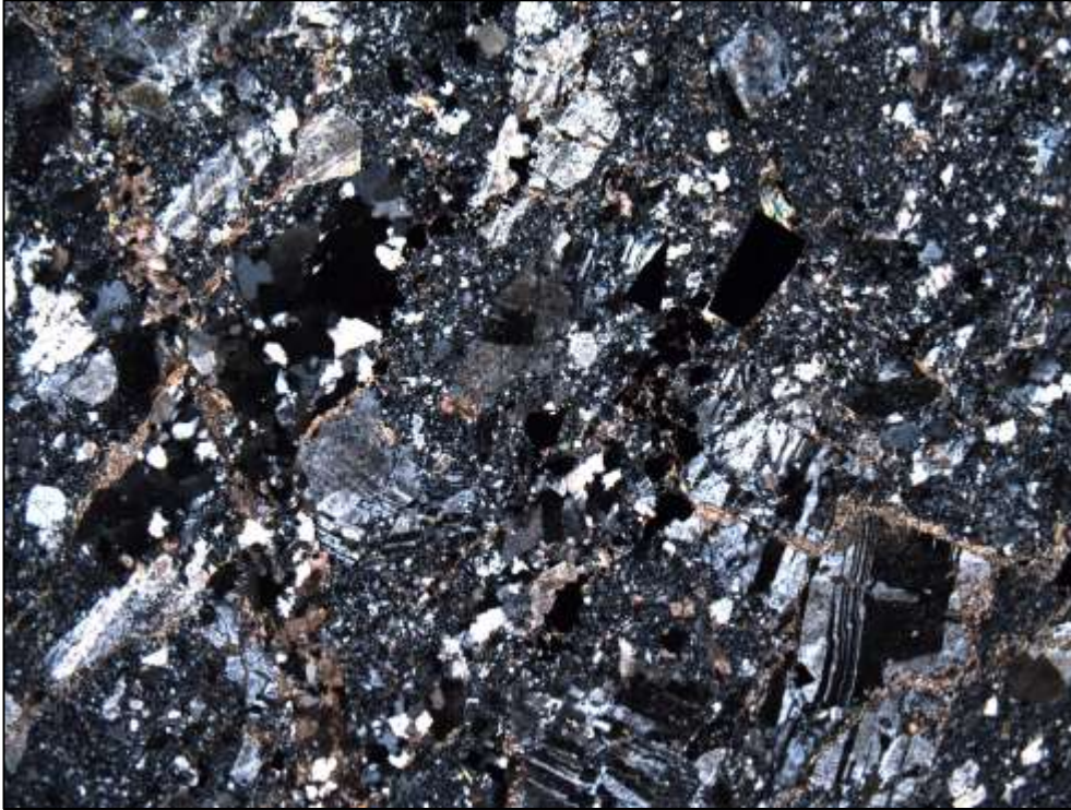
Fig. 9b. PMC-3, 111.4m. QF porphyry. Phenocrysts mainly plagioclase of various sizes, some cut by sericite-carbonate shears. Quartz phenos are small and minor. Crossed polars. Width of view = 5 mm.
