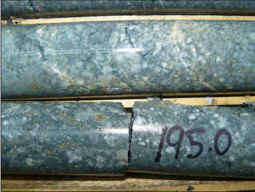
Fig. 12b. PMC-3, 195.0m. Litho sample of QF porphyry cut by sulfide veinlets. Sample contain 6.5 % Na 2 O, 0.71 % S, 0.30 % Cu and 0.01 % Mo. Petro sample at 194.8m (see Fig. 13).
