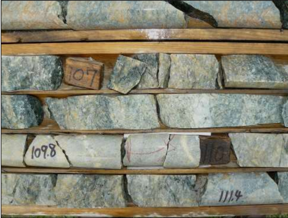
Fig. 9a. PMC-3, 109.8m. Litho sample of QF porphyry. The paler areas are due to increased amounts of fine-grained carbonate. Petro sample at 111.4m (see below).
