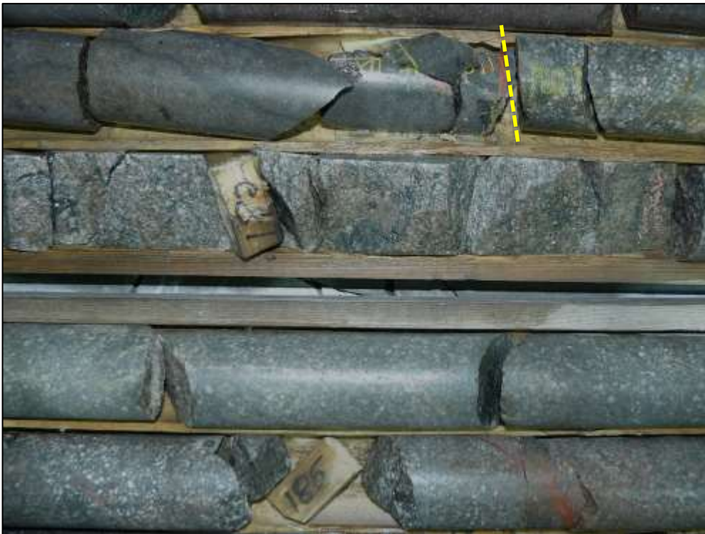
Fig. 26a. CR02-1. Contact at 180.7m (marked) between impure mafic rock and QF porphyry.
