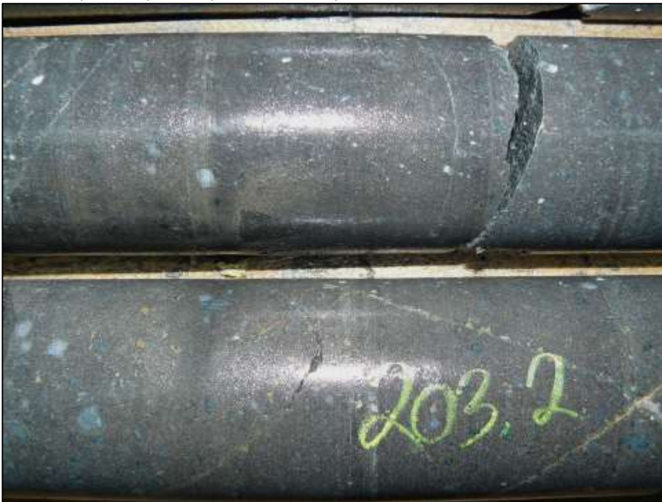
Fig. 27a. CR02-1, 203.2m. Litho sample of impure mafic rock. Although this lithology carries large quartz grains, it has the Mg and Cr contents of a mafic rock. The quartz grains may be xenocrysts.
