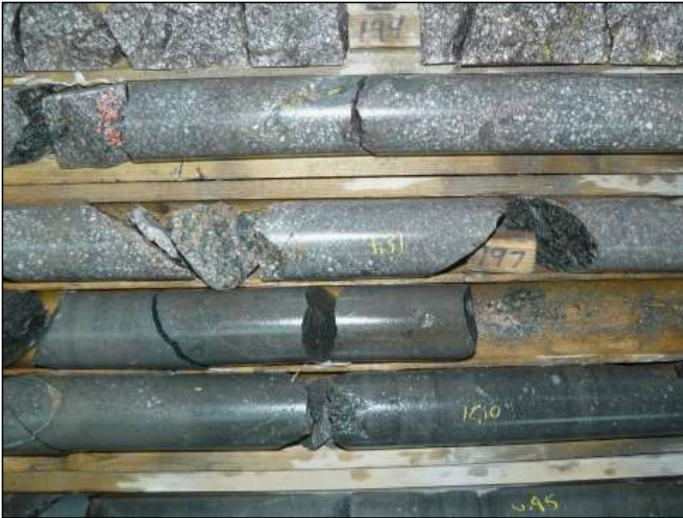
Fig. 26b. CR02-1. QF porphyry and impure mafic rock (contact is at 198.1m, just out of view). Note scattered phenocrysts of quartz and feldspar in the mafic rock.
