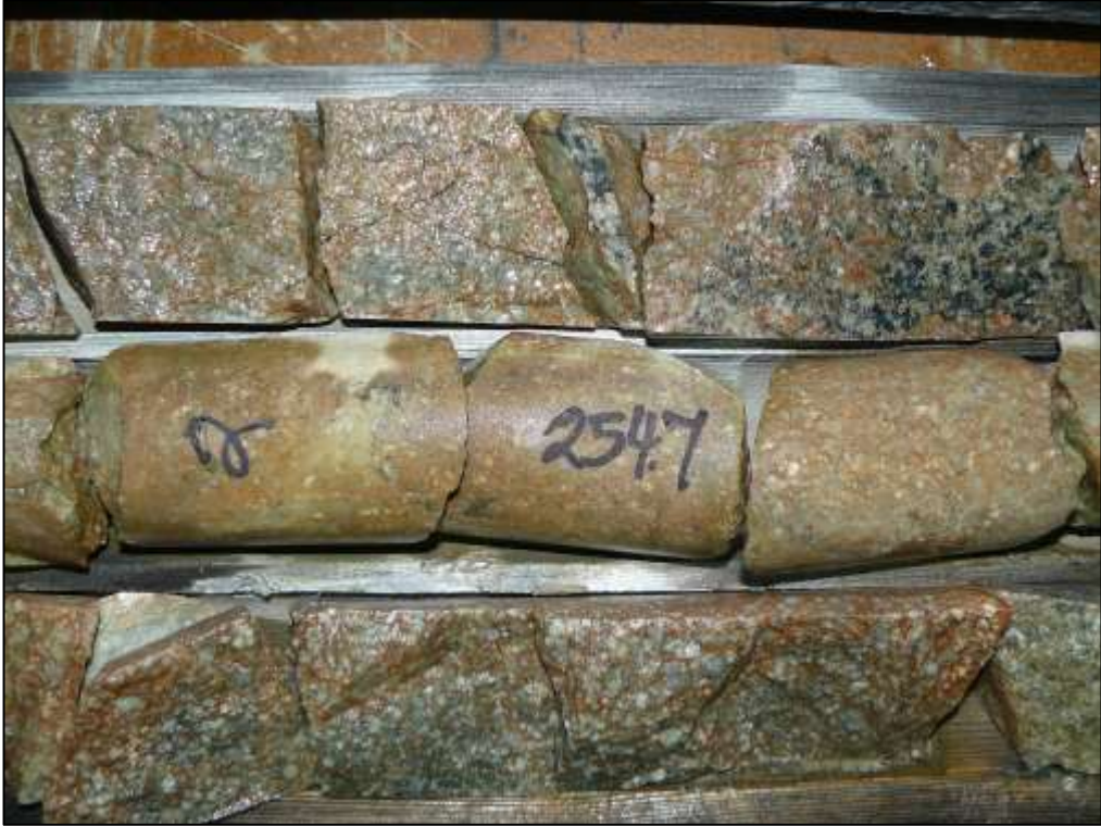
Fig. 30b. CR02-1, 254.7m. Litho sample of QF porphyry with 7.1 % Na 2 O, 0.62 % S and 0.09 % Cu.
