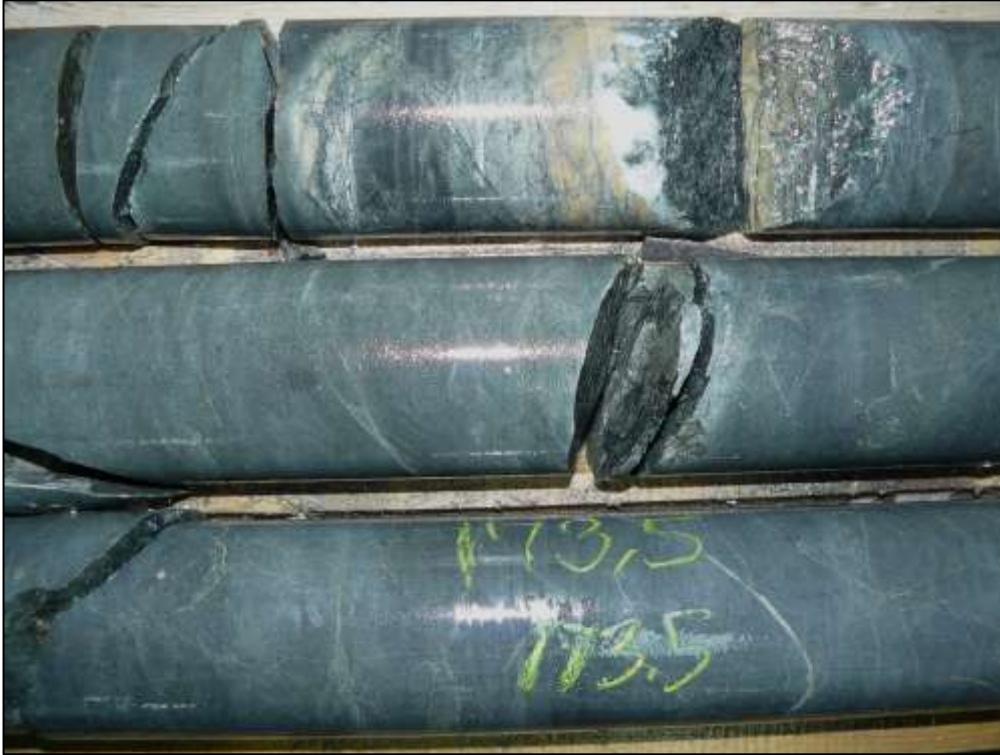
Fig. 25b. CR02-1, 173.5m. Litho sample of fine greywacke. Sample contains 0.23 % S and 0.08 % Cu.
