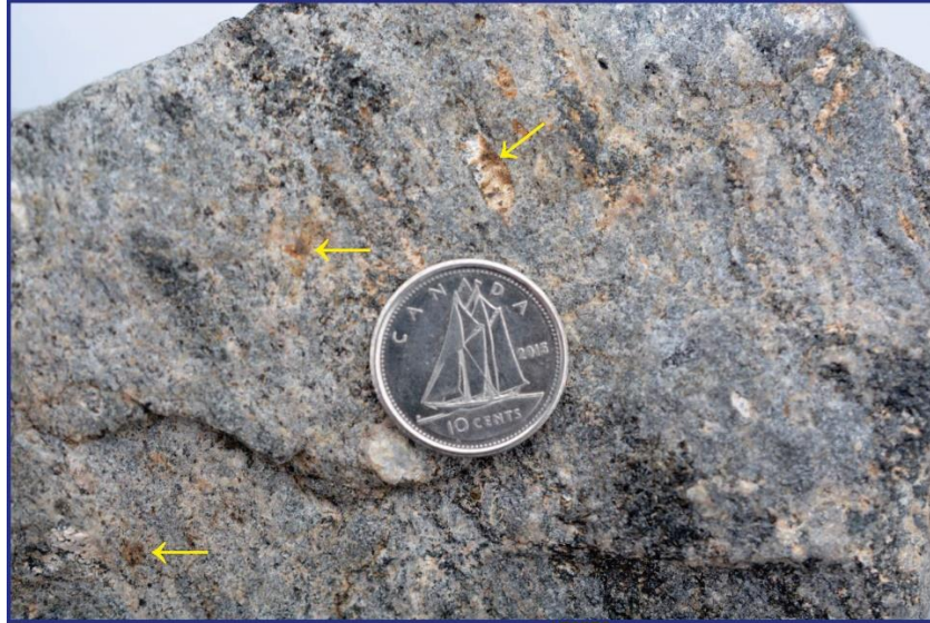
Photo 3. Biotite-clinopyroxene ijolite with magmatic foliation from site 72301, which contains 7.64 wt.% Total REE, 0.05 wt.% Nb, 0.18 wt.% Y, 0.93 wt.% Th, 94 ppm U, and 0.35 wt.% Ba. Arrows point to red-brown britholite. The larger crystal above the coin shows britholite altered to an unknown soft white mineral.
