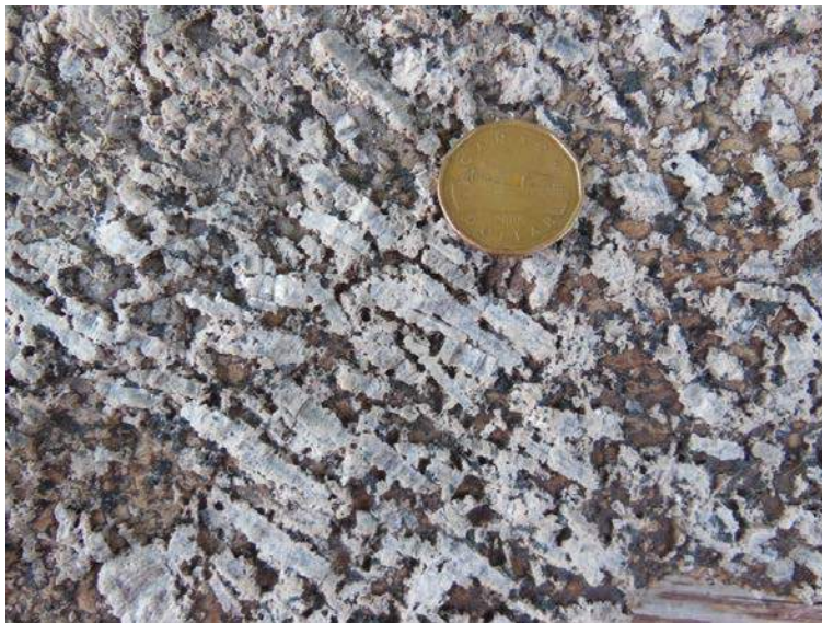
Photo 2. Nepheline syenite on the west side of Camp Lake that reveals a trachytic texture defined by oriented K-feldspar laths embedded in a recessive weathered nepheline-rich matrix that is stained orange by weathering. Dark green pyroxene grains occur within the nepheline-rich matrix.
