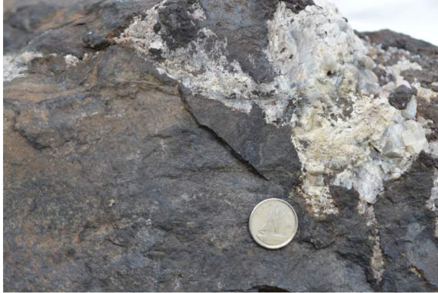
Photo 18: Magnetite-rich rock from old test pit cut by late silico-carbonatite masses that transect subtle magmatic layering at top left corner.
