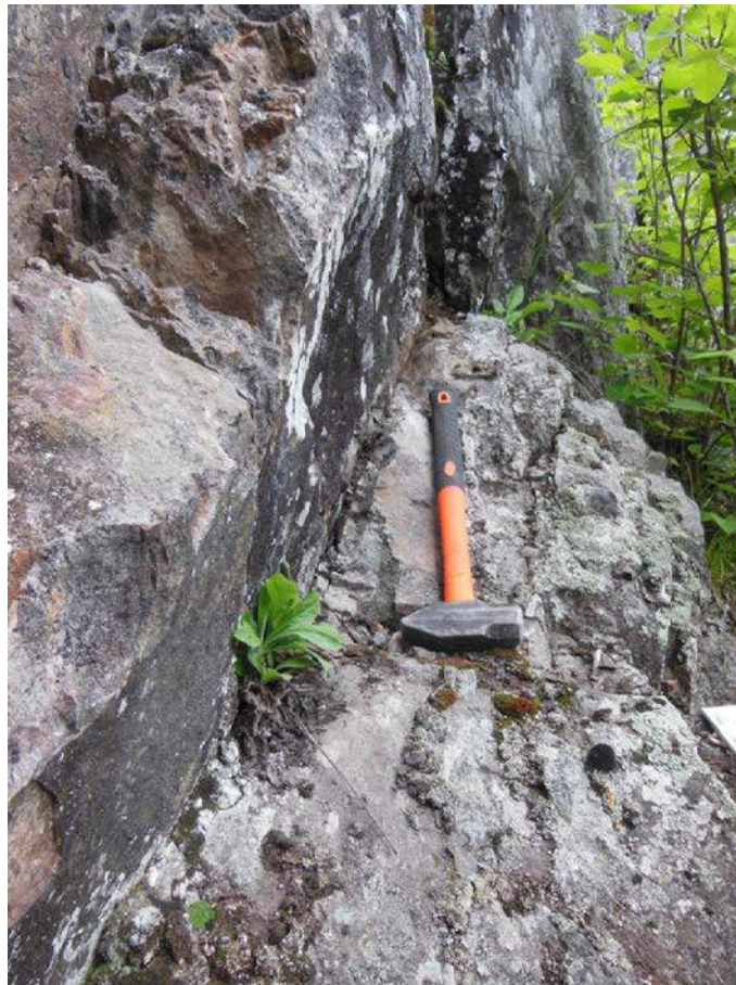
Photo 21. Altered pink apatite-magnetite-aegirine syenite at the base of the cliff which comprises the only in situ exposure of the Pole Lake REE-Ba-Th-Nb zone. Assay 1634565 represents a 70 cm chip sample across this zone in upper left corner that returned 3.4 wt. % \Sigma REE, 1514 ppm \Sigma HREE, 5005 ppm Th, and 2.62 wt.% Ba (Appendix 2). The zone is open in width as a large talus pile covers the mineralization to the right of the hammer.
