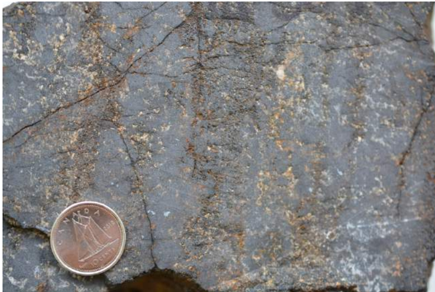
Photo 19. Subtly layered, magnetite-rich material from old pits near Camp Lake Road at UTM 340773E, 5294697N. The dark brown area is rich in magnetite and disseminated white fine- to medium-grained minerals consist of calcite, pyrochlore, barite, and nepheline. Chemical analysis 1634507: FeOT 61.4 wt.%, MgO 12.2 wt.%, Ba 1626 ppm, Cr 1161 ppm, Nb 894 ppm, Th 554 ppm, and Sc 97 ppm.
