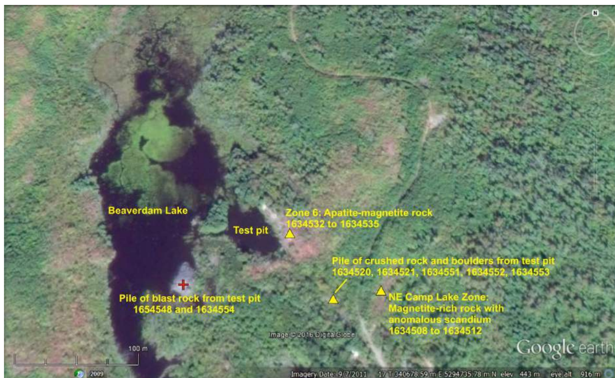
Figure 12. Locations of Zone 6 apatite-magnetite deposit on Beaverdam Lake and the NE Camp Lake magnetite zone. Numbers represent individual and ranges of assay samples in Appendix 2.
