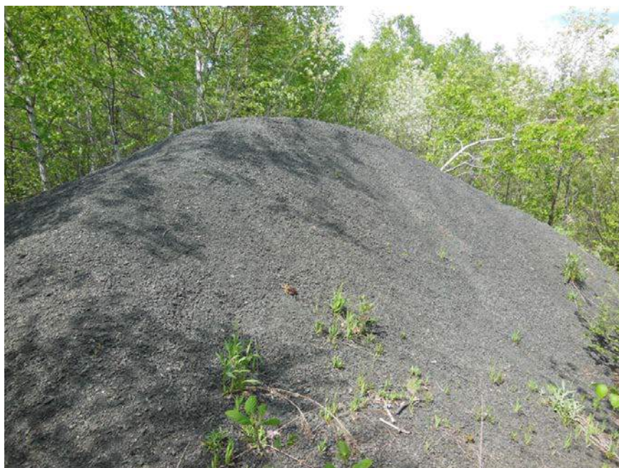
Photo 26. Pile of crushed magnetite-rich material from Multi-Minerals test pit at the Zone 6 apatite-magnetite deposit. Grab samples for assay were taken from three different parts of the pile (Appendix 1: 1634521, 1634522 and 1634551).
