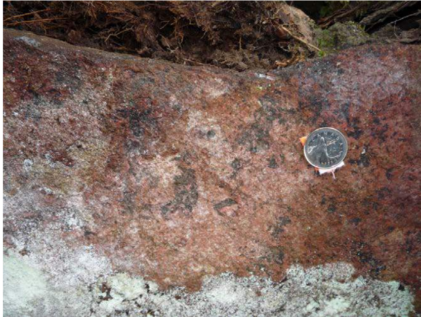
Photo 24. Fracture surface composed of brick-red natrolite, dark green clinopyroxene and niobium titanite hosted in ijolite near the Pole Lake REE-Ba-Th-Nb occurrence. The white area along the bottom consists of organic matter.
