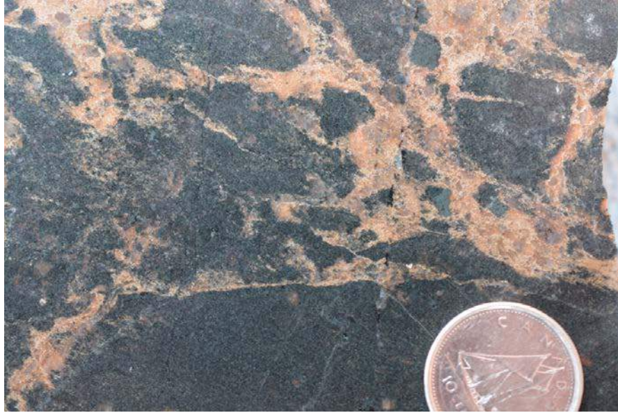
Photo 17. Niobium mineralization in ijolite breccia in boulder from a pile of blast material on Beaverdam Lake. The deep orange nepheline-rich matrix contains disseminations of masses of fine-grained, bronze coloured pyrochlore. The highest values for following elements obtained from this sample (1634554): Nb 1.73 wt.%, Ta 647 ppm, and U 754 ppm. Thorium is elevated at 2516 ppm but total REE is relatively low at 933 ppm.
