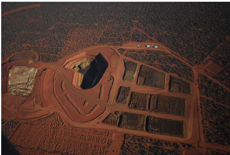
Photo 1. Example of an open pit rare earth mine in carbonatite laterite at Mount Weld, Australia of Lynas Corporation that is the highest grade REE deposit currently known at 11.2 wt.% \Sigma REO (Castor and Hedrick 2006). Photo from https://www.lynascorp.com/Pages/How-are-Rare-Earths-Mined.aspx
