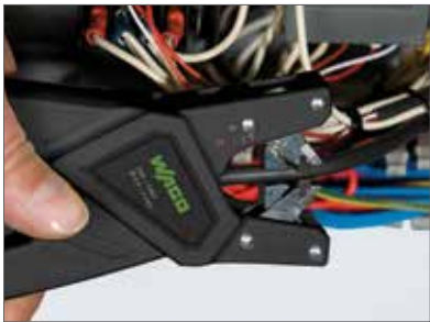
Automatic stripping for control and sensor wires
