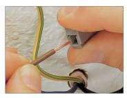
**Connection:** Squeeze connector housing and insert stripped conductor into square entry, then release
