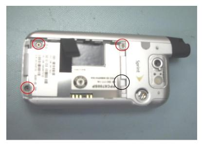
9.2.4 Use removed battery cover to place screws on, so none will be lost
