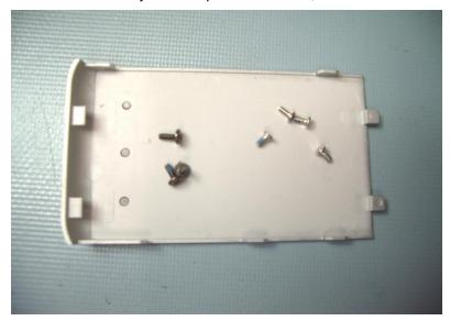
9.2.5 Remove camera module cover by lifting up and left
