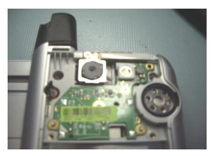
9.4.3 Replace camera module cover by pushing down and to the right over speaker. Secure the two cover screws with 1.5 mm Phillips screw driver
