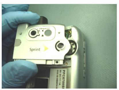
9.2.6 Pull camera module circuit board up and out towards top of device, ensuring that it is separated from its connector directly vertical, without twisting
