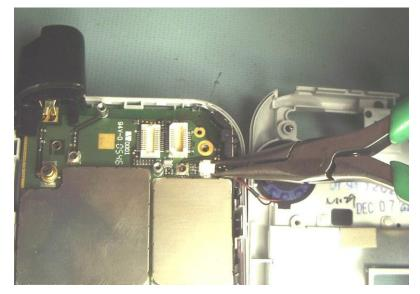
9.2.11 Disconnect the keypad connector pin in the bottom left corner from the main circuit board
