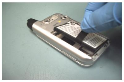
9.2.3 Using Torx power screw driver, remove two primary case screws, starting from bottom left to top left. Using 1.5 mm Phillips screw driver remove two camera module screws, starting from top right to bottom right. Removal of the final camera module screw will destroy Warranty dot cover. It will be replaced during re-assembly
