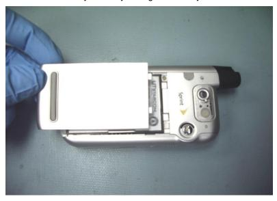
9.2.2 Remove battery by pulling lifter tab out
