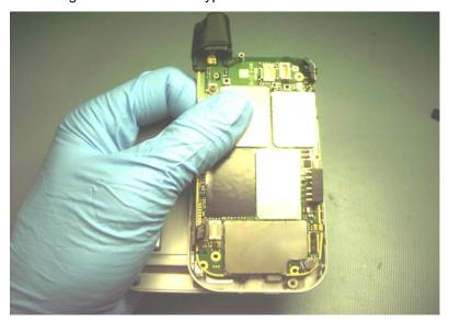
9.4.2 Replace camera module circuit board and camera lens piece, taking care to reinsert them vertically like steps 9.2.7 and 9.2.8
