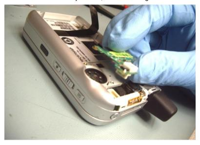
9.2.7 Disconnect camera lens piece from it's connector in the same fashion, being careful to lift it out vertically
