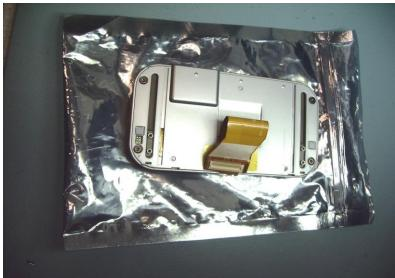
9.3.3 Attach LCD connector to Main Circuit board. Remove static dissipater mesh from anti static anti dust cohesion cloth and reapply it around LCD connector on main circuit board
