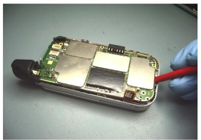
9.2.13 Lift the main circuit board up and to the right. Pry the LCD connector and static dissipater mesh apart from the main circuit board with the main pry tool
