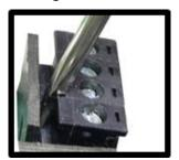
When removing the connector use the screw driver as shown above to avoid pin damage.
