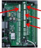
Using the wiring diagrams and terminal descriptions at the end of this manual wire up the terminals for the I/O board located on the terminal Board
