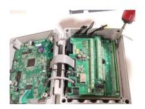
1. Install and tighten 4 mounting screws for the shield plate and board stack.
