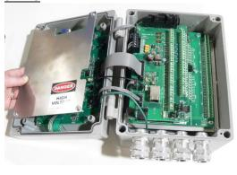
1. Replace the Door Shield with the 4 screws you removed earlier.
