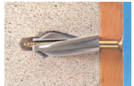
Fig. 19: Minimum screw length.
