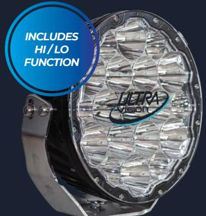
The Nitro 180 sets an entirely new standard for performance in LED driving lights achieving 1 lux at 1.8km. In addition a Hi/Lo function reduces the power to 30% for more built-up areas or when approaching traffic is still a long way off. The Nitro 180 is fitted with the same proven stainless steel bracket as the Nitro 140 and is supplied complete with a wiring harness, Hi/Lo switch, polycarbonate lens cover and anti-theft.
