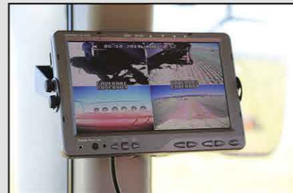
Tractor - The side post is a great location to mount your monitor. Cables may be tucked between the pillar and the window
