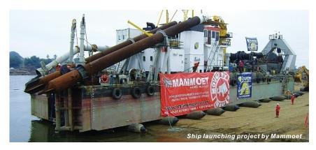
BUODER marine airbags can be used for ship launching/landing, marine salvage, and heavy lifting. All marine airbags are made by innovative holistic wrapping technology. Manufactured and tested comply with ISO 14409 standard.
