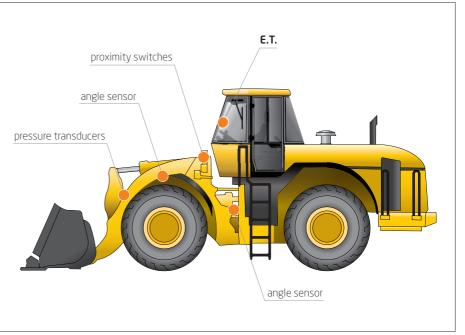
Accuracy: 0÷2% with one transducer Accuracy: 0÷1% with two transducers
