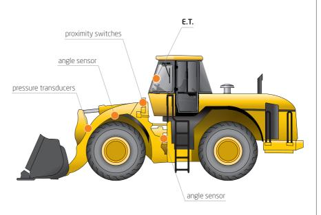
Accuracy: **0÷2% with one transducer** Accuracy: **0÷1% with two transducers**
