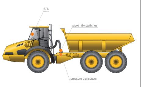
Accuracy: **0**÷**3**% with well-balanced load
