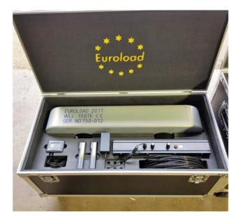
The above picture shows a 300 and 150 tonne telemetry load link. Fitted with a ELT-24 transmitter, the options for the customer are endless. Powered from 2 off AA batteries to give exceptional usage time. The load cell has Euroloads standard screw off battery cover giving a ingress protection of IP68.
