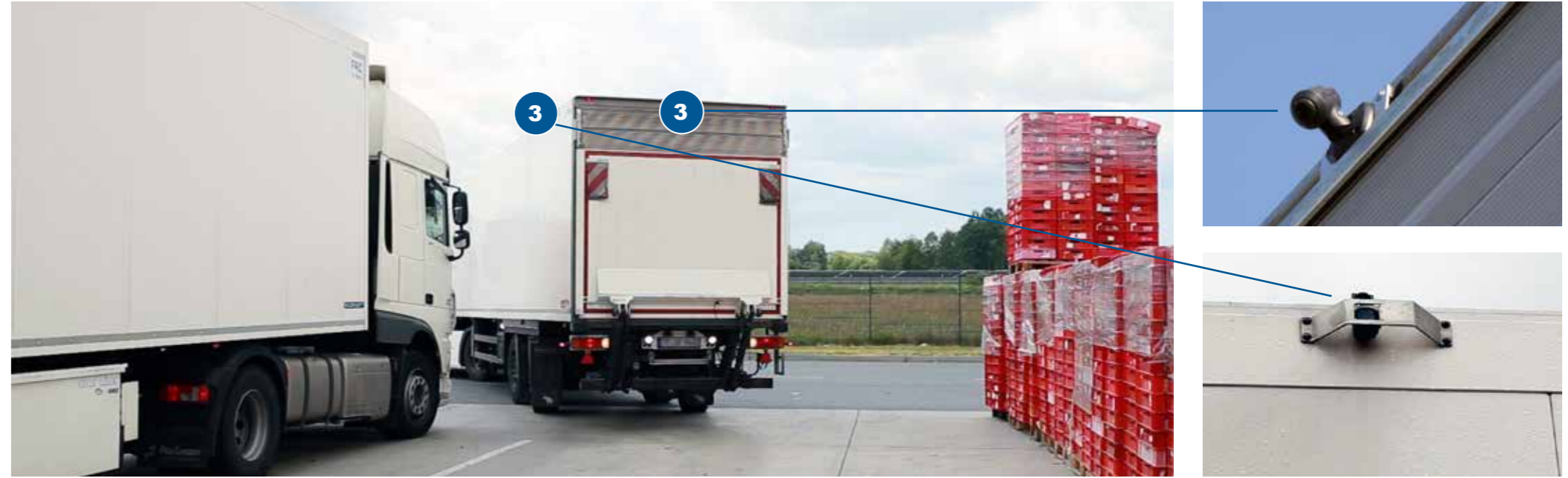
Installation positions of the MVS cameras. Sides and rear for 270° birdseye view.
