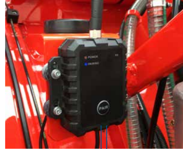
Digital wireless system with a maximum range of 120 meters.
