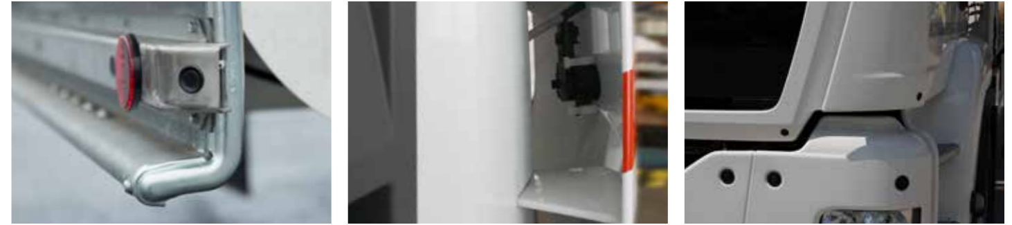
Installation examples for ultrasonic sensors. Left: Rear bumper Centre: Front bumper (inside) Right: Front bumper
