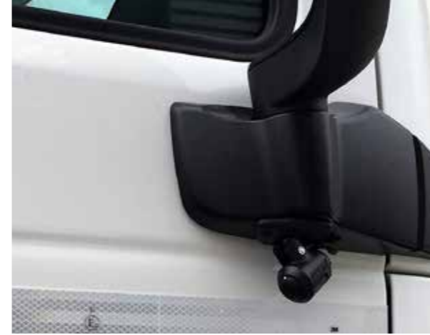
Side room monitoring for safe right turn.
