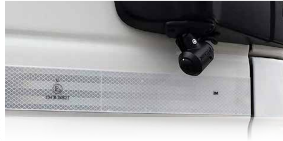
Heavy-duty camera installed on the tractor unit to increase visibility when making turns right.
