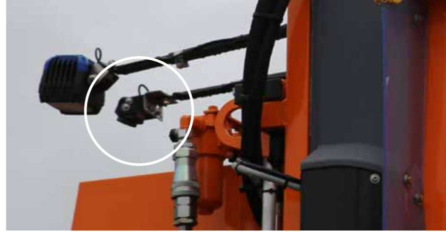
Heavy-duty cameras for monitoring the vehicle's rear and operating area as well as the vehicle's sides.
