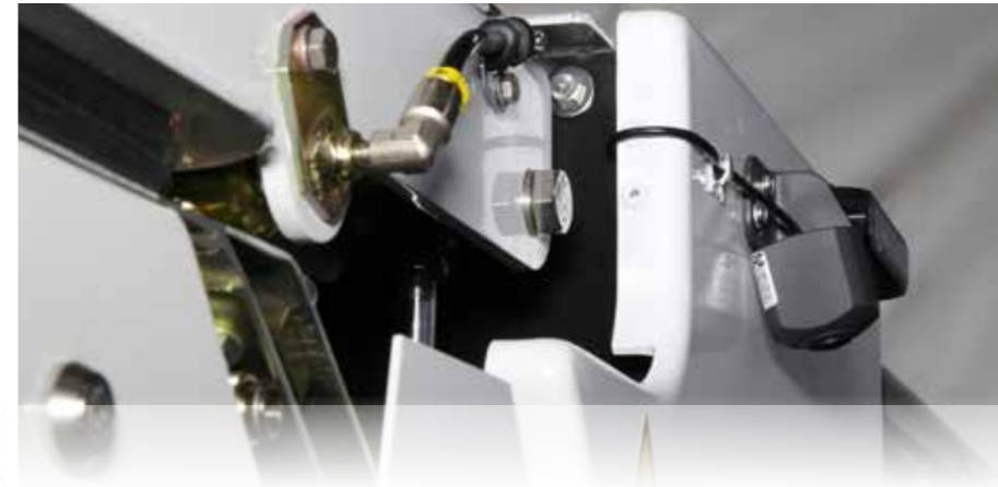
There are 4 cameras installed around the vehicle allow for a 360° birdseye view.
