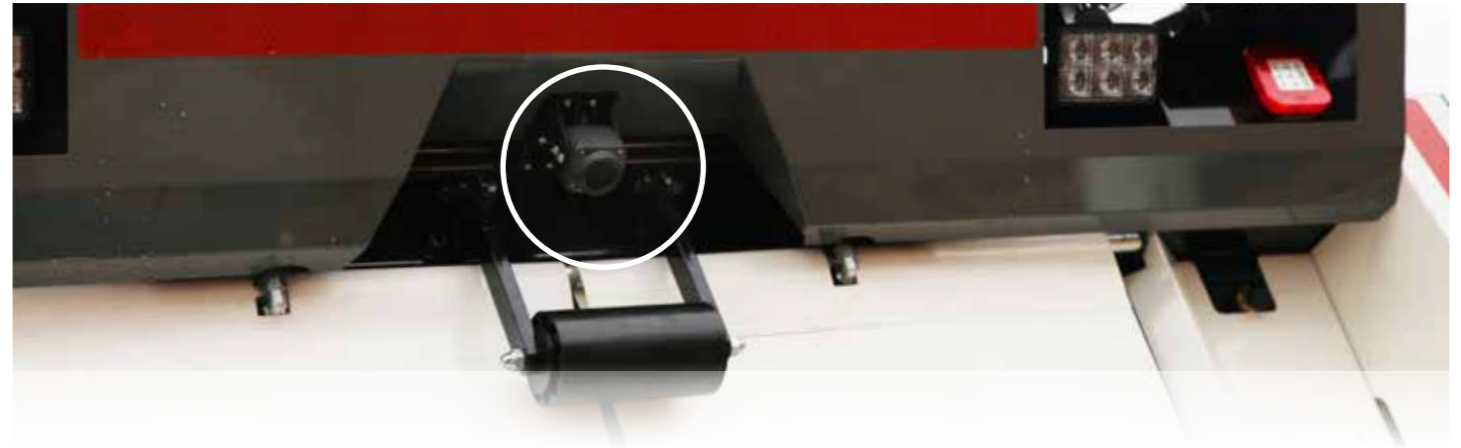
Refuse collection vehicles with camera for monitoring the front area of the vehicle. Heavy-duty camera for monitoring the rear and operating areas.
