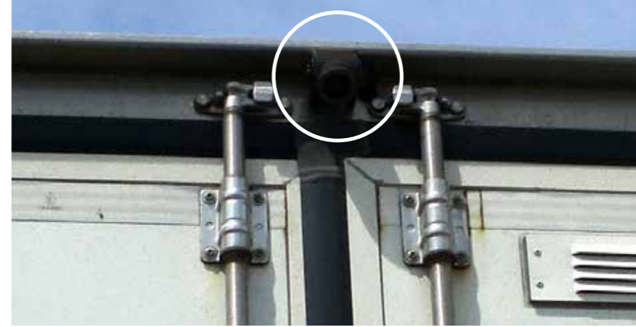
Semi-trailer truck with heavy-duty camera above the portal to monitor the rear area of the vehicle.
