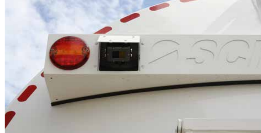
Tankers with heavy-duty camera to monitor the rear area of the vehicle.
