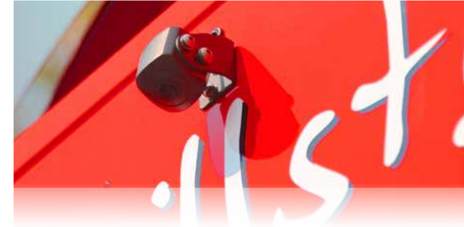
There are 4 cameras installed around the vehicle allow for a 360° birdseye view.
