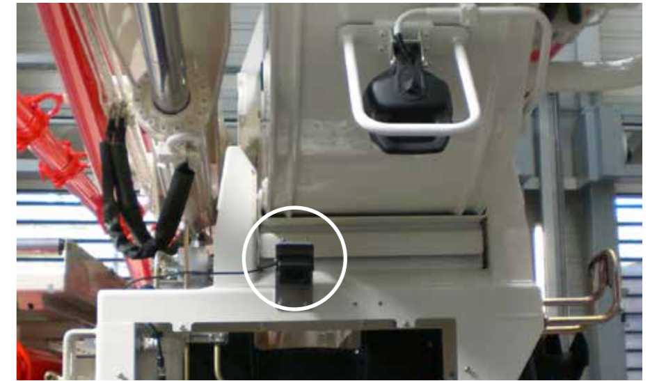
Motec MC3000B camera at the rear of a concrete-mixing truck.
