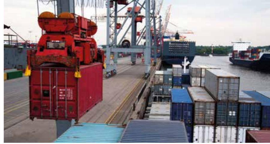
Rail-bound mobile harbour crane handling containers.
