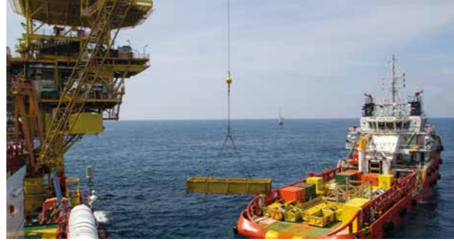
Offshore structure on open sea. Camera and monitor systems provide more precision in crane movements.
