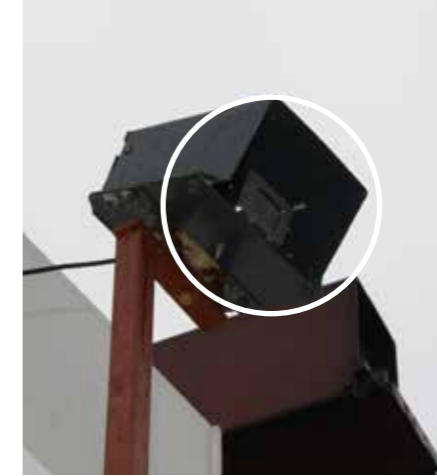
Stationary "Pirate X" cutter suction dredger off the coast of Lower Saxony. Fitted with a Motec camera and monitor system for monitoring cable winch winding, for example.
