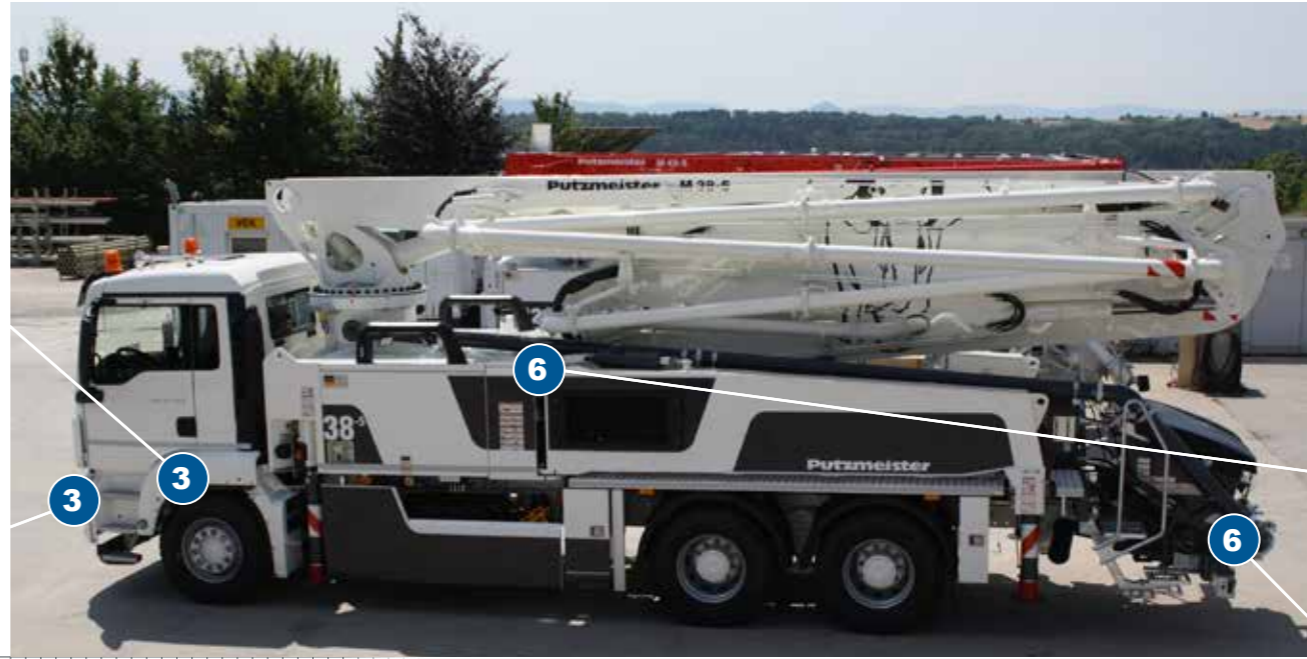
Putzmeister concrete pump truck with front camera, ultrasound and radar sensor, side monitoring and rear space monitoring.
