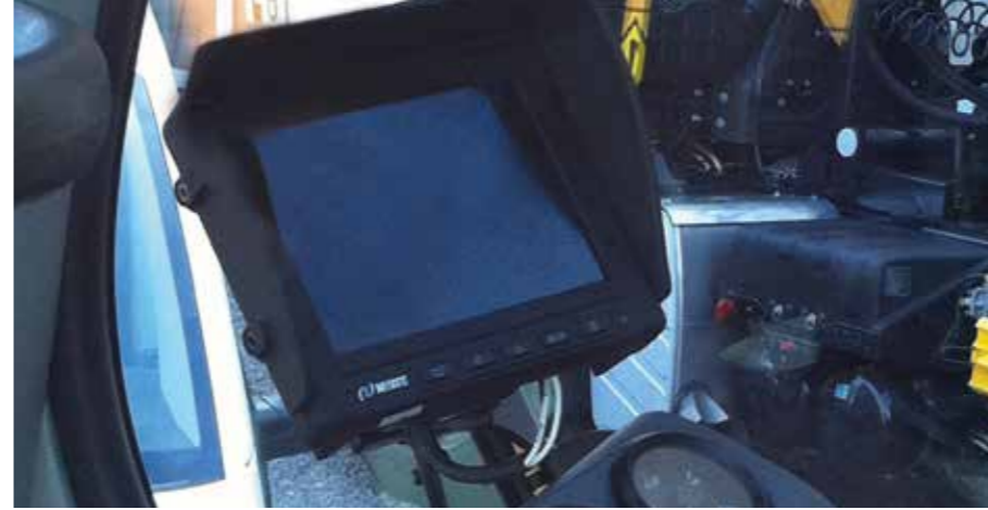
Front-end loader with the MD3071A heavy-duty monitor for rear-space monitoring. The display provides a crystal clear representation of the camera images.
