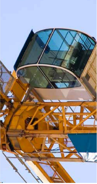
Detail view of a top-slewing tower crane with cabin. The motor zoom camera and the radio transmitter are mounted at the crane carriage.
