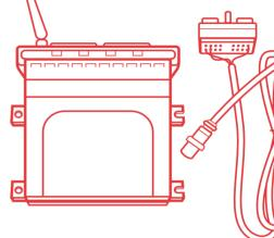
The System is tested for operation at 5Kv, to ensure a margin for most machine and install applications. It will not detect low voltage under 1,000 volts with consistency or predictability for ensuring safe working distances.
