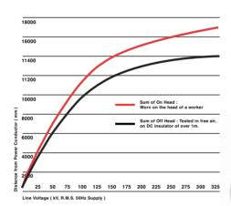
The Capacitive sensing system allows the eLert Electrical Safety Helmet sensor to detect live conductors even if there is no current flowing.
