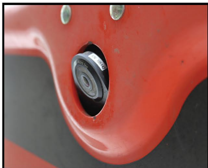
Custom kit includes bracket that utilizes existing buzzer hole on specific Bobcat models
