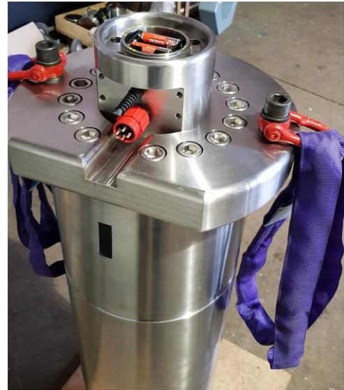
Euroload Limited have supplied a load monitoring pin to our exclusive Dutch agent Eurorope Nederland BV for their Van Beest 1250 Tonne sling saver shackle. Euroload replaced the existing pin with our fully stainless steel load pin, down hole dual strain gauged, IP67, telemetry and cabled output, heavy duty electronic housing, screw off battery cover .
