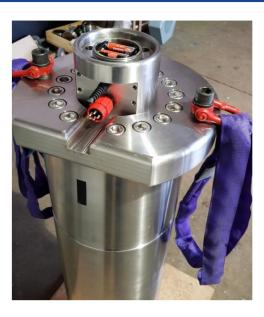
Euroload Limited have supplied a load monitoring pin to our exclusive Dutch agent Eurorope Nederland BV for there Van Beest 1250 Tonne sling saver shackle. Euroload replaced the existing pin with our fully stainless steel load pin, down hole dual strain gauged, IP67, telemetry and cabled output, heavy duty electronic housing, screw off battery cover.
