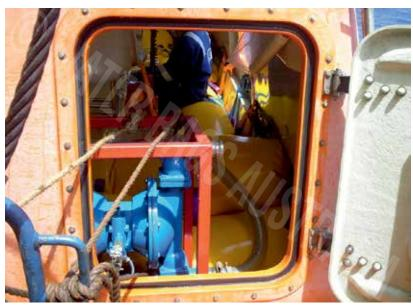
16 x LBT-375kg lifeboat test water bags used in an enclosed lifeboat
