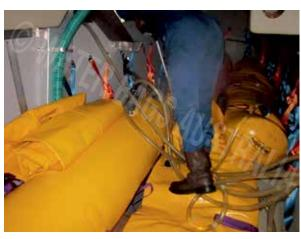
LBT-375 lifeboat water bags working inside the totally enclosed lifeboat
