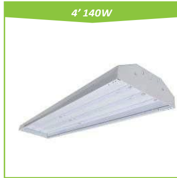
Item#: HDS-BL-LHB-4811-140W-850D 4' LED Linear High Bay Fixture Power 140W Width:11" Lens: Optional Voltage Input: 100-277V ac Lumens: 15000 lm Certificate: ETL/cETL, DLC
