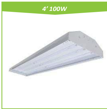
Item#: HDS-BL-LHB-4811-100W-850D 4' LED Linear High Bay Fixture Power 100W Width:11" Lens: Optional Voltage Input: 100-277V ac Lumens: 11000 lm Certificate: ETL/cETL, DLC
