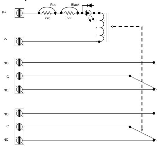
The ASRB-1 uses a 5 VDC relay. Resistance in series with the relay is needed to alleviate stress on the relay and LED when higher voltages are applied.
