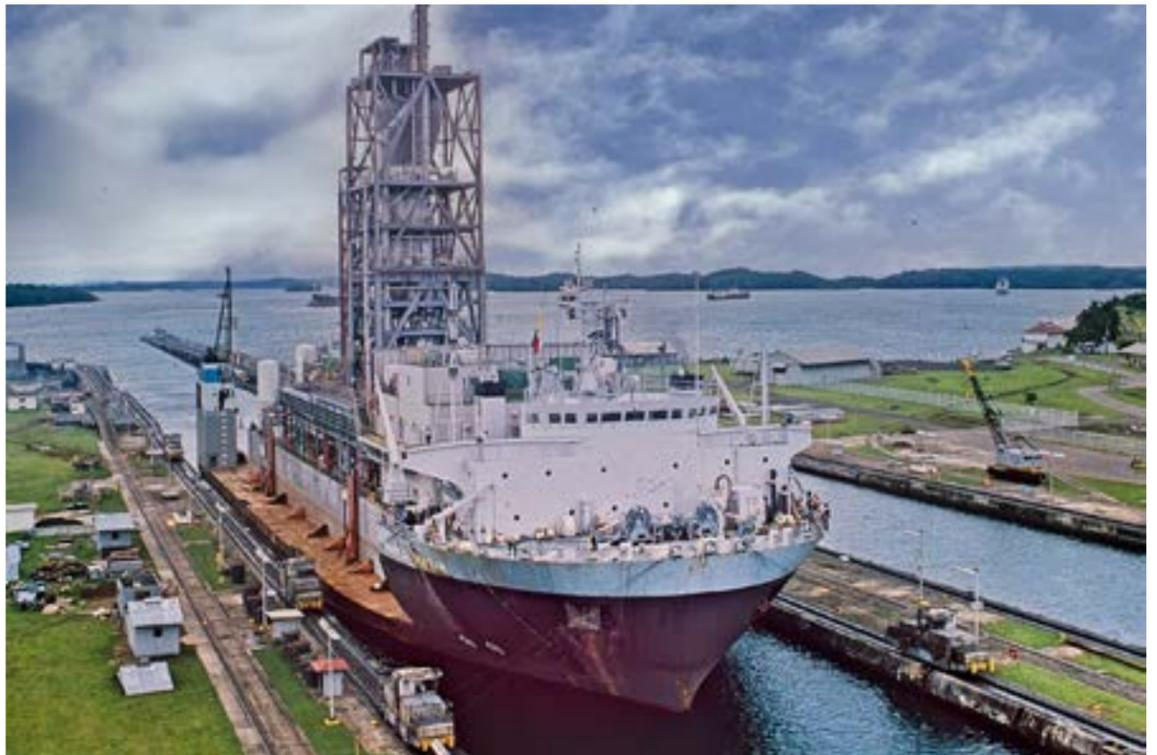
Chemical plant on a barge going thru the Panama Canal
