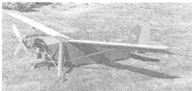
The grand-daddy of aerial target radio-controlled aircraft. The OQ-2, dating to 1939, had a span of 12 ft., fuselage length of 8.6 ft., gross weight of 108 pounds and achieved a speed of 90 mph. The Radioplane Company manufactured the aircraft with a metal frame triangular fuselage and wooden wings which were fabric-covered. Note the concentrically shafted counter-rotating propellers employed to eliminate engine torque effects. Engine was an opposed twin 2-cycle developing 6.5 horsepower manufactured by the Righter Company. (Photo by the author.)
