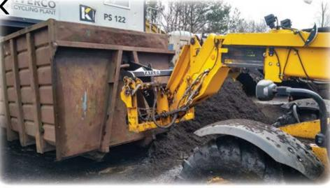
Commonly used in green waste and recycling industries for a speedy and safe way of moving empty 'roll on-roll off' skips. We've been told these save huge amounts of time and costs compared to using the lorries to manoeuvre the skips.
