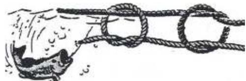
**Timber Hitch** - Used in hauling timber and for commencing the diagonal lashing. Pass the end of the rope around the timber. Bring it up and around the standing part, then twist it back about itself two or more times. The weight of the timber will hold it securely.
