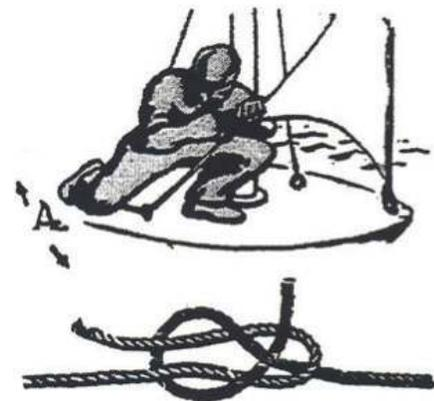
**The Sheepshank** - This knot is valuable for taking up a slack when both ends of the rope are tied, or for strengthening a weakened rope. Gather up the amount to be shortened, then make a half hitch around each of the bends.
