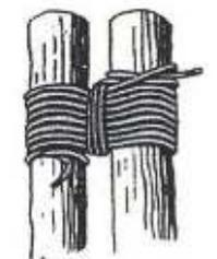
**Continuous Lashing** - Continuous lashing holds small sticks at right angles to long sticks and is useful in making table tops, seats, etc. Follow these steps in laying a table top.
