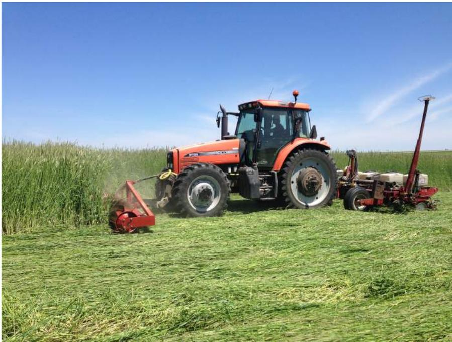
Figure 1. Front-mounted roller-crimper used to terminate cover crops and to create mulches.
