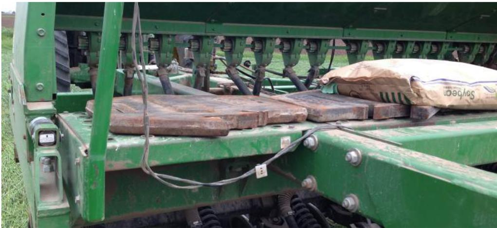
*Adding weights to the planter can help ensure good seed-to-soil contact and good stand establishment*
