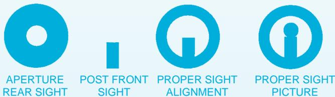
The rear sight has a small hole that the shooter must look or peep through. The front sight is usually a post sight. When looking through the round peep hole, the eye automatically centres the front sight in the centre of the rear peep- at the strongest point of light. The target sits on top of the front post.
