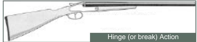
A hinge action firearm opens or “breaks” in the centre, similar to the movement of a door hinge. To open the action, the release handle is pushed to one side and the barrel or barrels are pressed downward. The used shell is then ejected, new shells are inserted manually and the barrel is closed. This is a common type of action in shotguns.
