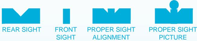
Most factory-ordered rifles are equipped with an open rear sight and a "bead" or "post" front. The top of the bead or post should be centered within the rear sight and placed on the bottom of the target.
