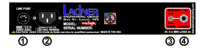
1 – FUSE- This is the line fuse for the amplifier. The proper fuse should be installed as indicated on the rear panel of the unit. The table below shows the proper fuse to be used with the indicated line voltage. NOTE: Failure to install the proper fuse based on the line voltage noted can result in personal injury, fire, damage to the amplifier or other nasty things too numerous to mention here.
