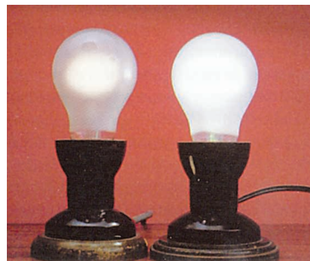
Figure 33. The bulb on left side has higher resistance, so its power is less. It glows less brightly. The bulb on right side has less resistance, so its power is more. It glows much more brightly.
