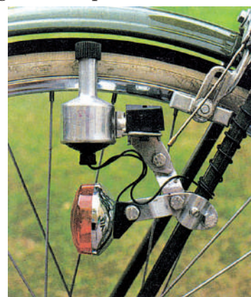
Figure 34. The bicycle dynamo in this picture also uses a rotating magnet inside a fixed coil of wire.
