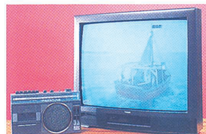
(c) Radios and televisions work only with d.c. (They have a device in them which converts a.c. supplied to them into d.c.).
