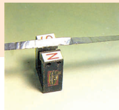
Figure 22. In this photograph we can see a piece of aluminium foil that has been fixed between the poles of a strong magnet. When a current is passed through the foil, it is pushed upwards, away from the magnet. It happens due to repulsion between the two magnetic fields : one from the magnet and one from current.
