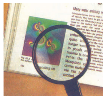
Figure 35. A convex lens being used as a magnifying glass to read the small print of a book.
