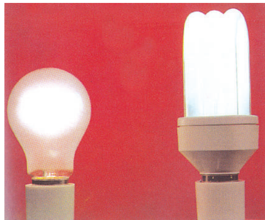
Figure 41. The bulb shown on the left side is the traditional, filament-type bulb. This is not energy efficient because it wastes a lot of electric energy as heat. The bulb shown on the right side is called Compact Fluorescent Lamp (CFL) which is energy efficient because it consumes much less electric energy. This is because it wastes much less electric energy as heat.
