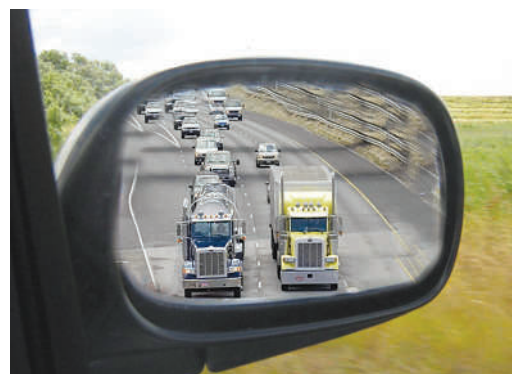
Figure 52. Convex mirror is used as a rear view mirror (or side view mirror) in vehicles.
