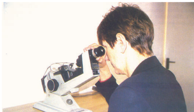
Figure 49. An optician measuring the power of a spectacle lens by using an instrument called diopmeter.
