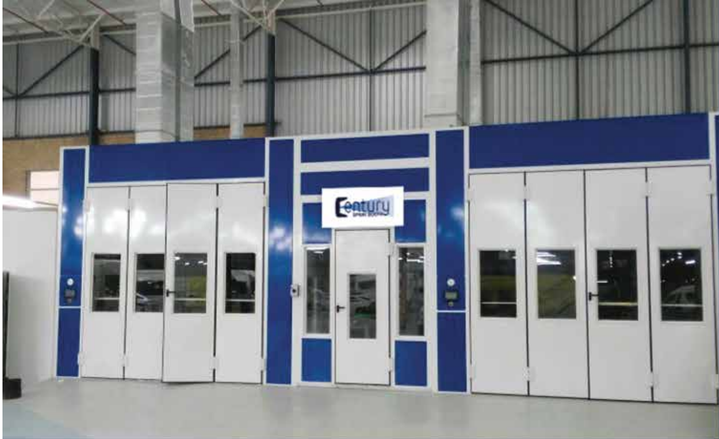
Two Spray Booths with Mix Room in between
