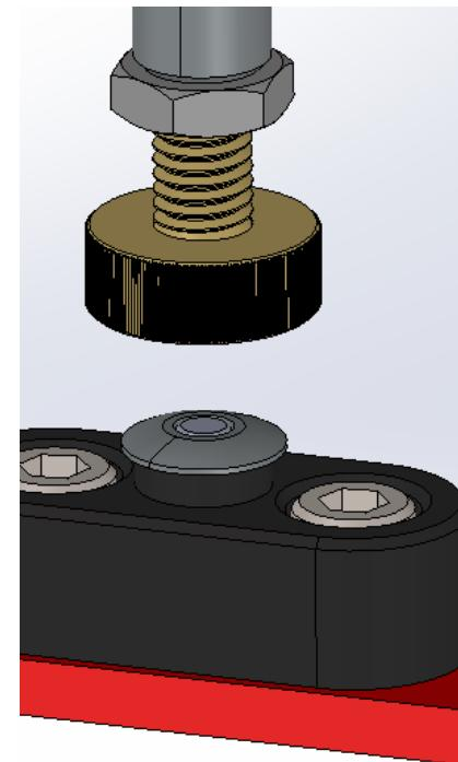
Press the primer into Primer Insert until the press has no more travel. This will set the primer to the correct depth and not put excessive force on the primer
