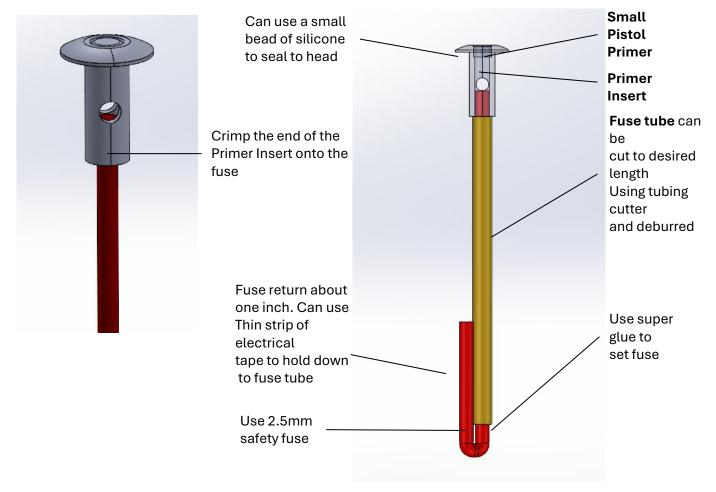
Fuse tube is set with red Loctite
