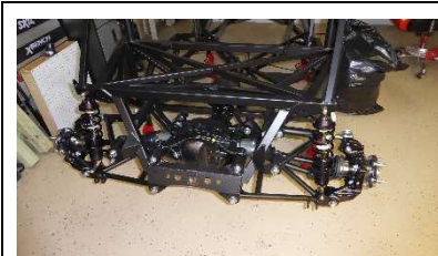
0818-31: Rear Shocks Installed.
