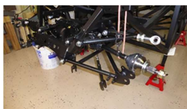
0818-29: CV Axles Installed.
