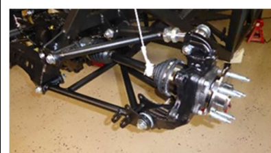
0818-30: Spindles and Hubs Installed.
