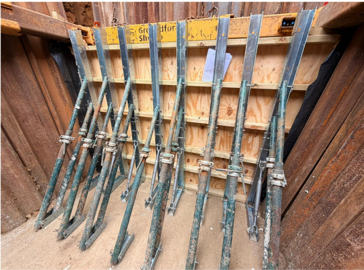
Super-Form Large Bracket, joined with large Upright for 2m pour height
