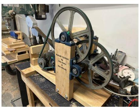
apparatus failed. The original wood carriage was made with pine and was nailed together. I'm surprised it lasted this long.
