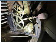
The original bell ringing system in the church steeple was a swinging or pealing bell design. Basically, the bell was mounted on a swinging yoke and when someone would pull a rope it would start the bell swinging back and forth, the clapper would strike the bell rim and create the ringing. At some point
