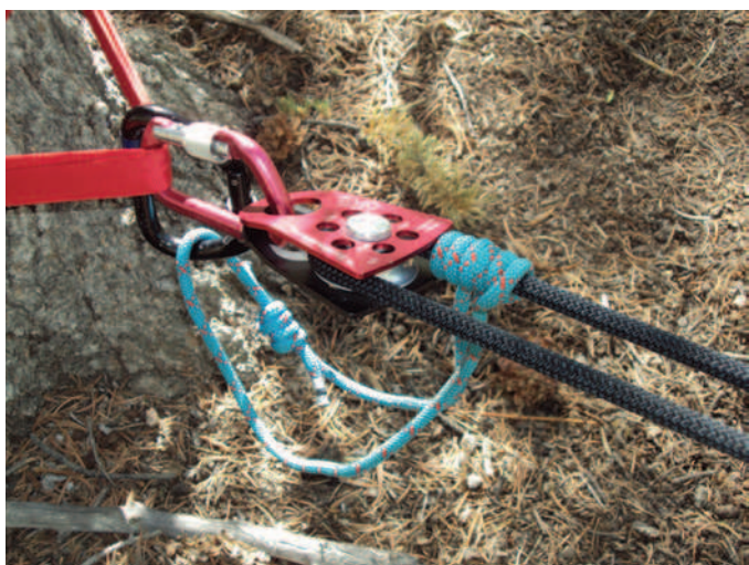
FIGURE 56-22 Prusik-minding pulley. The haul system can only move the load a certain distance before it needs to be reset. Before resetting the system, the Prusik is “set” to grip the rope and holds the load, taking tension off the haul system so that it can be reset. The Prusik will also set automatically, preventing the load from being dropped if there is a failure in the haul system. (Courtesy Loui H. McCurley.)
