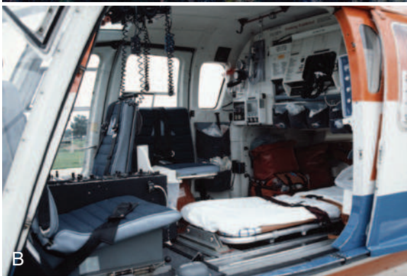
FIGURE 58-23 A , The BO-105, historically a workhorse of the U.S. air medical transport fleet, was often equipped with high-skid landing gear that facilitated landing on unimproved surfaces. B , Interior of the BO-105 depicts positioning of the patient stretcher and crew seats and gives an idea of patient care space in a light-twin helicopter. (Courtesy Stephen H. Thomas.)
