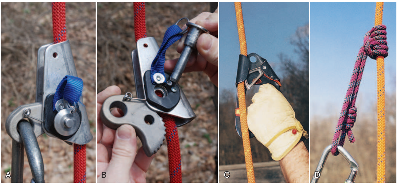
FIGURE 55-25 A, Gibbs ascender applied to rope. When the device has been assembled and attached to the rope and the eye of the cam is pulled, the cam squeezes the rope and holds fast. When the cam is released, the device can be moved along the rope. B, Gibbs ascender dismantled with shell around rope. Note cam (lower left) and pin (upper right). C, Clog-handled ascender. Although used where climbing a fixed rope is required, handled ascenders are rarely used in rescue. D, A three-wrap Prusik hitch can sometimes be used in lieu of a mechanical ascender. (Courtesy DC Copper.)
