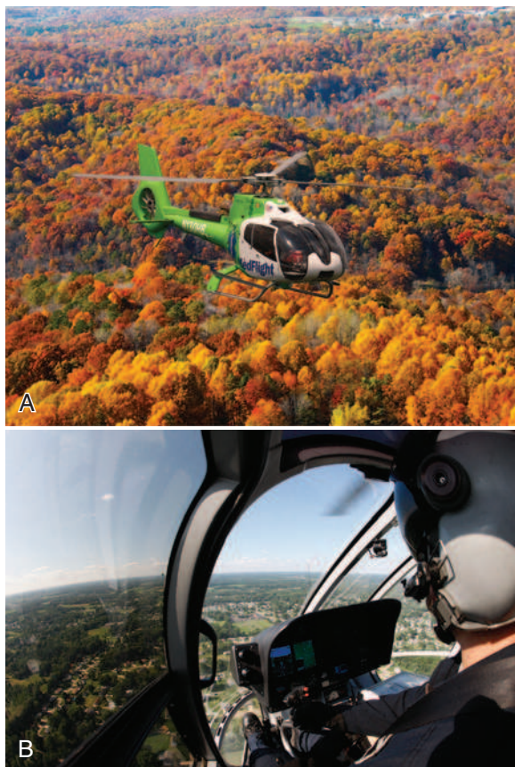
FIGURE 58-12 The Airbus EC130 (A) is noteworthy for superb visibility from the pilot's seat (B). (Courtesy MedFlight of Ohio.)
