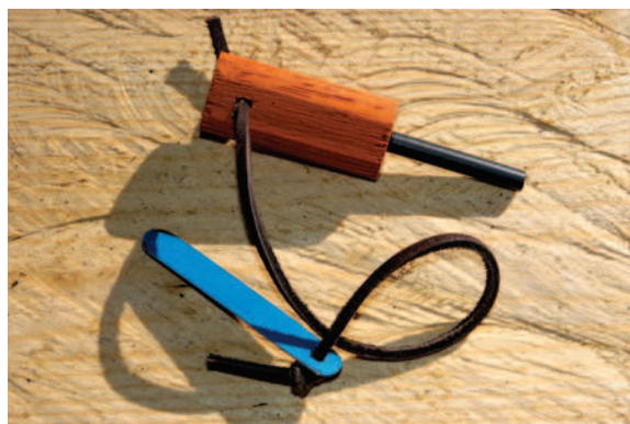
FIGURE 59-32 Metal match with a hacksaw blade scraper.
