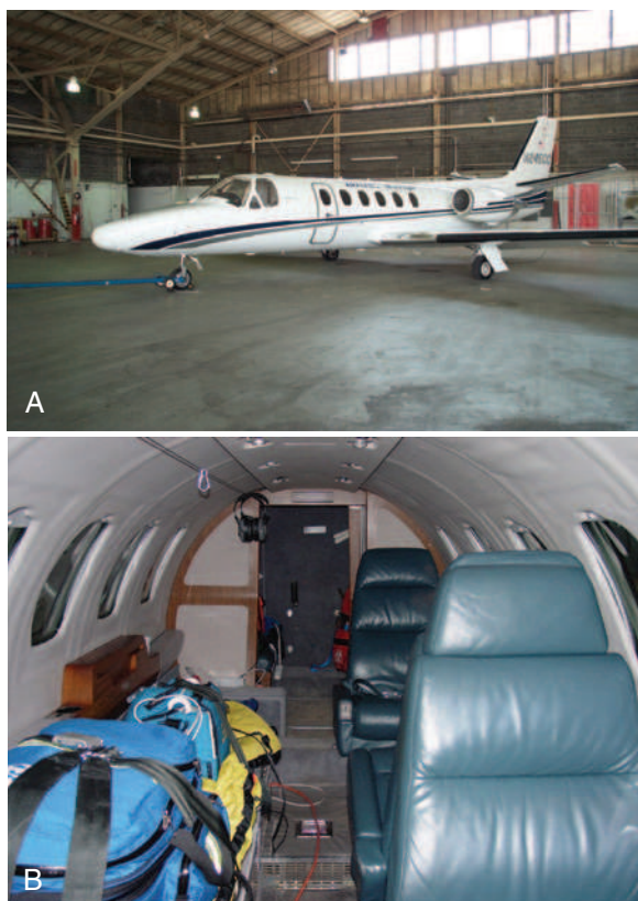
FIGURE 58-7 A, The Cessna CitationJet III is typical of intermediate-range air medical transport jets. B, Interior of the Cessna CitationJet III depicts a layout characteristic of intermediate-range air medical transport jets. (Courtesy Boston MedFlight.)
