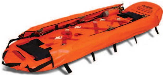
FIGURE 57-28 Life Support International’s Rescue Sled (manufactured by Switlik) is a unique, durable, and inflatable device that provides 102 kg (225 lb) of buoyancy and weighs under 9 kg (20 lb). Shown is the Rescue Sled with integral flotation devices inflated (one tube each side). (Courtesy Life Support International, Inc.)
