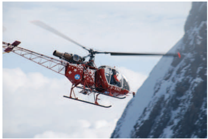
FIGURE 56-33 Aerospatiale Lama helicopter operated by Air Zermatt, Switzerland. The Lama has limited aeromedical capabilities, but is capable of rescue at altitudes of more than 4000 m (13,100 feet). (Courtesy Ken Zafren.)
