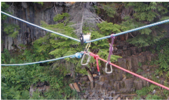
FIGURE 56-27 Highline. A special highline pulley can be used to decrease friction. The rescue load (not shown) hangs from the pulley. The lines on either side of the rescue load are tag lines that are used to pull the load along the highline. (Courtesy Loui H. McCurley.)
