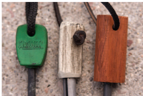
FIGURE 59-30 Metal match handles. From left to right: plastic, synthetic antler, and wood.
