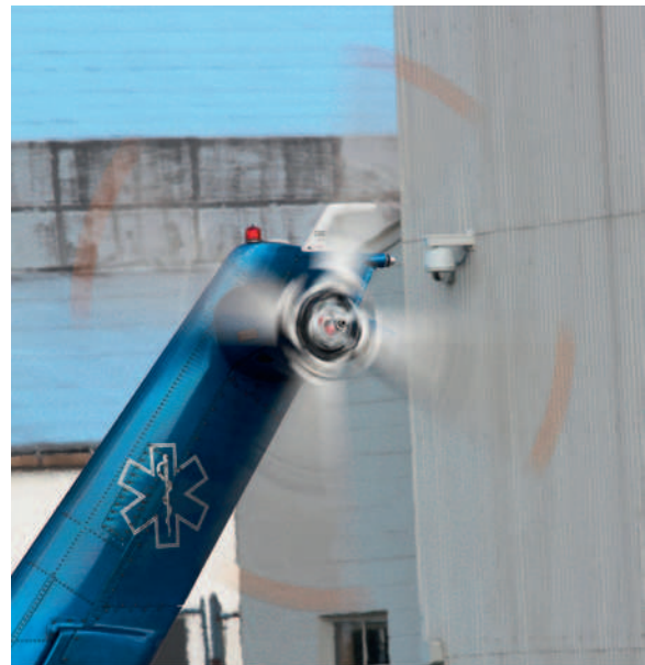
FIGURE 58-37 A spinning tail rotor is virtually invisible. (Courtesy Boston MedFlight.)
