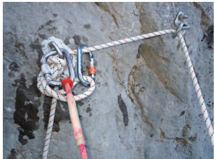
FIGURE 56-42 Knot block in a closed system. A knot block is placed against a glue-in bolt and secured with a carabiner (left). After removing the lanyard (pink rope), the canyoneer can descend on the opposite strand (right). (Courtesy Giacomo Strapazzon.)
