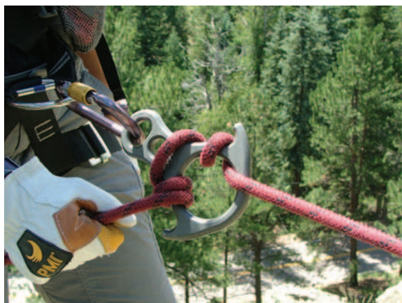
FIGURE 56-15 Double wrapped figure-eight ascender. The double wrap increases friction, enabling control of a rescue load. (Courtesy Loui H. McCurley.)
