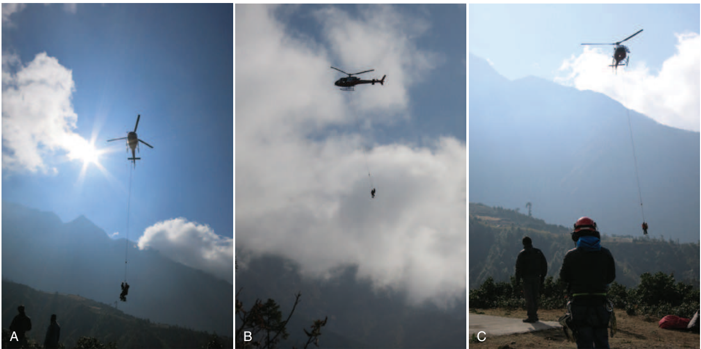
FIGURE 58-42 A long-line device can be used for a “short-haul” of a patient (A) from the rescue site for a short distance (B) to a stabilization area (C). (Courtesy Monika Brodmann Maeder.)
