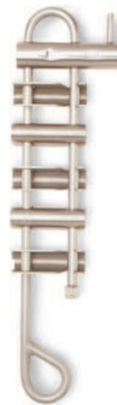
FIGURE 55-24 SMC National Fire Protection Association brake bar rack. Straight frame shown; frame also available with eye twisted 90 degrees. The top bar has been modified to allow a secure tie-off. (Copyright CMC Rescue.)
