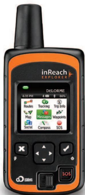
FIGURE 55-3 The DeLorme inReach Explorer satellite communicator allows remote tracking of its location, sends and receives 160-character text messages with GPS coordinates to cell numbers and email addresses worldwide, confirms delivery of messages, and has powerful navigation features, including an on-screen map view (14.8 × 6.2 × 2.6 cm, 190 g). (Courtesy of DeLorme, a Garmin Brand.)
