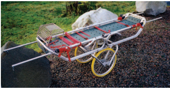
FIGURE 57-30 MacInnes Mk 6 Mountain Rescue Stretcher. Note the extending handles, folding head guard, and optional twin (solid) tires. (Courtesy MacInnes Rescue Stretchers.)
