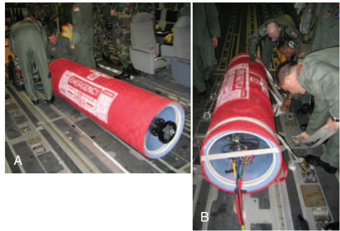
FIGURE 58-29 Cabin space is not an issue for medical transport in large airplanes, in which many patient interventions can be provided during flight. A , Hyperlyte portable hyperbaric chamber being inflated and rigged for a dive aboard a U.S. Air Force C-17 aircraft. At the time this photograph was taken, the aircraft was flying at 4572 m (15,000 feet). B , Hyperlyte portable hyperbaric chamber being secured to the deck of a U.S. Air Force C-17 aircraft. Note the gas lines feeding into the near end of the chamber. (Courtesy Robert C. Allen.)
