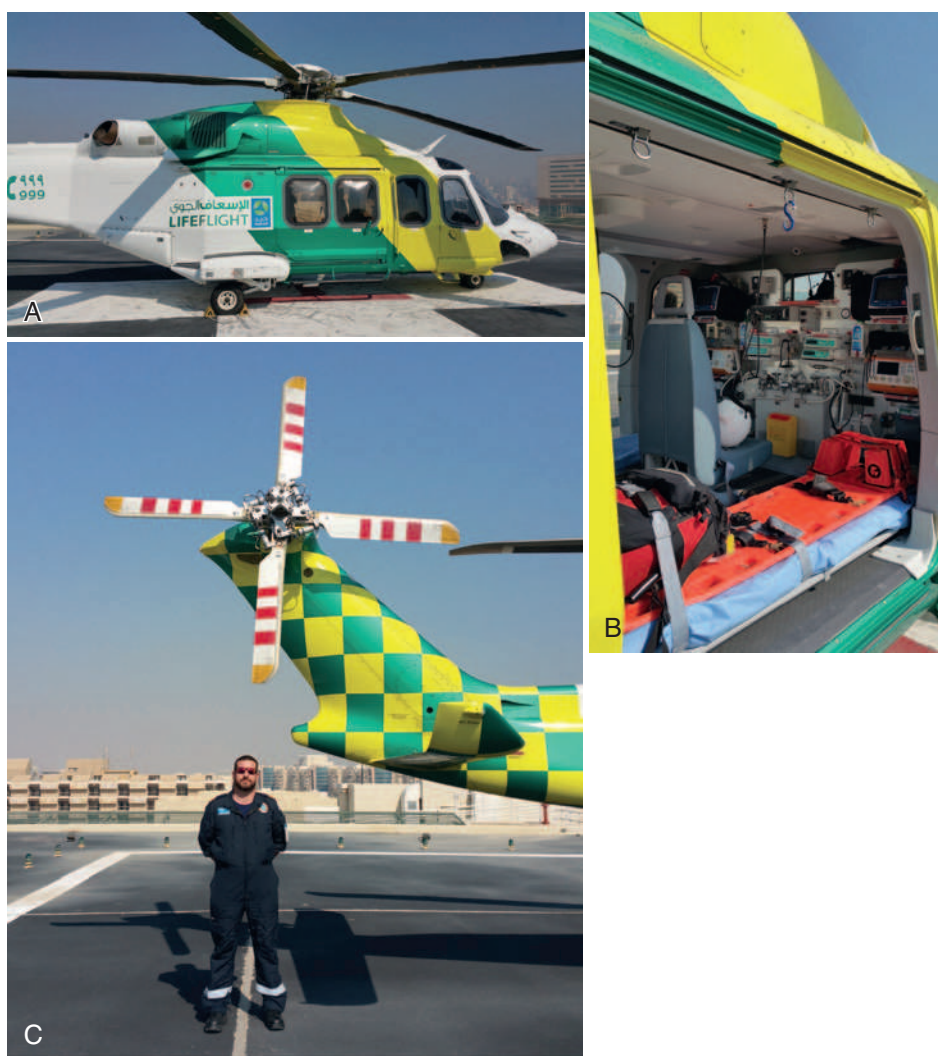
FIGURE 58-16 A , The AgustaWestland 139 is one of the larger aircraft used for civilian helicopter emergency services. Its size, speed, and range make it ideal for a number of mission types. B , Forward-facing view of the AgustaWestland 139 interior depicts typical layout for a fore-and-aft stretcher on each side of the cabin, with crew seating in between. Each stretcher has its own associated monitor, ventilator, and other medical equipment. C , The AgustaWestland 139 tail rotor’s placement offers an increased safety margin. However, in certain wilderness settings (e.g., desert) the aircraft’s weight causes settling in soft landing surfaces, and the tail rotor can become a hazard. (Courtesy Hamad Medical Corporation.)
