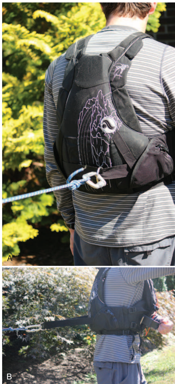
FIGURE 62-3 A and B, Life jacket with built-in rescue harness. It is essential for swiftwater use. (Courtesy Henderson McGinnis, MD.)
