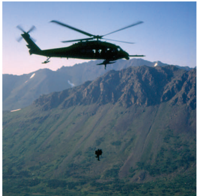
FIGURE 56-37 Pave Hawk hoist operation. The Pave Hawk is a version of the Black Hawk helicopter that is especially equipped for rescue operations. Shown here are two rescuers who are about to be inserted into a rescue scene. (Courtesy Ken Zafren.)
