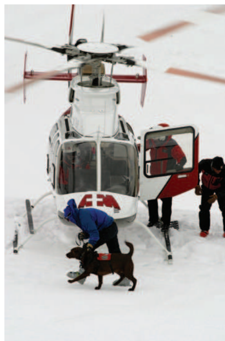
FIGURE 58-28 Helicopters have unique capabilities to work closely with ground-based teams, such as those executing avalanche search and rescue. Among the environmental factors that the crew must keep in mind is the drop in temperature inside the aircraft when sitting in a cold environment, which is an important issue when the aircraft is parked at higher (colder) altitudes. (Courtesy of Eric Swenson and University of Utah AirMed.)
