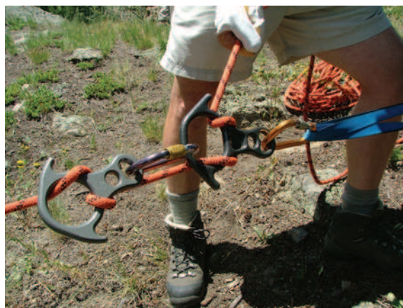
FIGURE 56-16 Stacked figure-eight brake. The two figure-eight brakes can be stacked using a carabiner (as shown) or webbing to provide enough friction to control a rescue load. (Courtesy Loui H. McCurley.)
