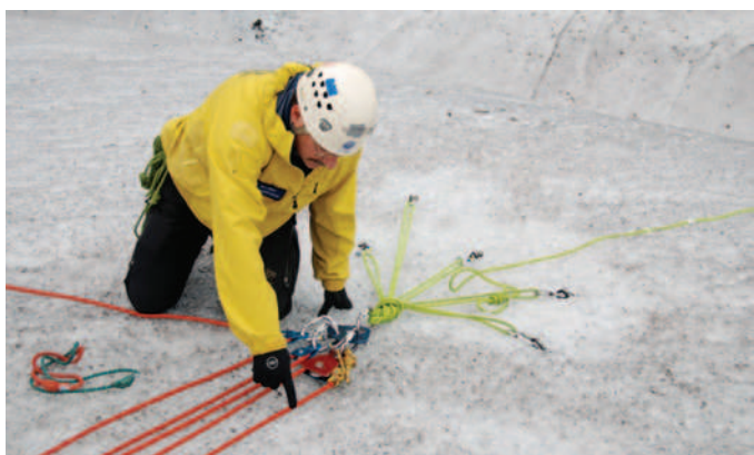
FIGURE 56-23 Five-to-one advantage haul system on a glacier. Note the load-sharing anchor. The pulley closest to the rescuer is a direction-change pulley that allows the rescuers to pull parallel to the crevasse from which they plan to raise the subject in a litter. (Courtesy Ken Zafren.)
