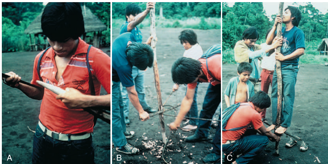
FIGURE 60-15 A, Young man sharpening a stick to a point. B, Lashing a cross-member to a pole. C, Standing on the pole to take measurements of the depth of penetration into the airstrip. (Courtesy John Walden.)
