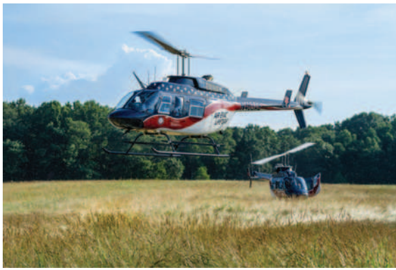
FIGURE 58-2 The Bell 206 LongRanger family has an extensive history of air medical use in civilian and military settings. Skid landing gear facilitates helicopter landing on nonpaved surfaces. (Courtesy Air Evac Lifeteam, Inc.)
