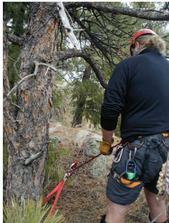
FIGURE 56-26 Friction brake load lowering. The rescuer is using a friction brake to lower a rescue load down a vertical face. (Courtesy Loui H. McCurley.)
