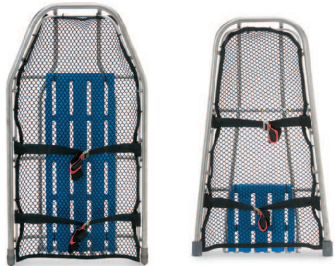
FIGURE 57-19 Split-apart rescue litter. The two parts of this type of litter can be nested, one on top of the other, and packed into the backcountry. The two pieces “hinge” together at the bottom, and are secured by integral threaded collars on the top rail that lock into place, eliminating the need for pins. The stainless steel version weighs 16 kg (35 lb), and the titanium version weighs 7.26 kg (16 lb). (Courtesy CMC Rescue, Inc.)
