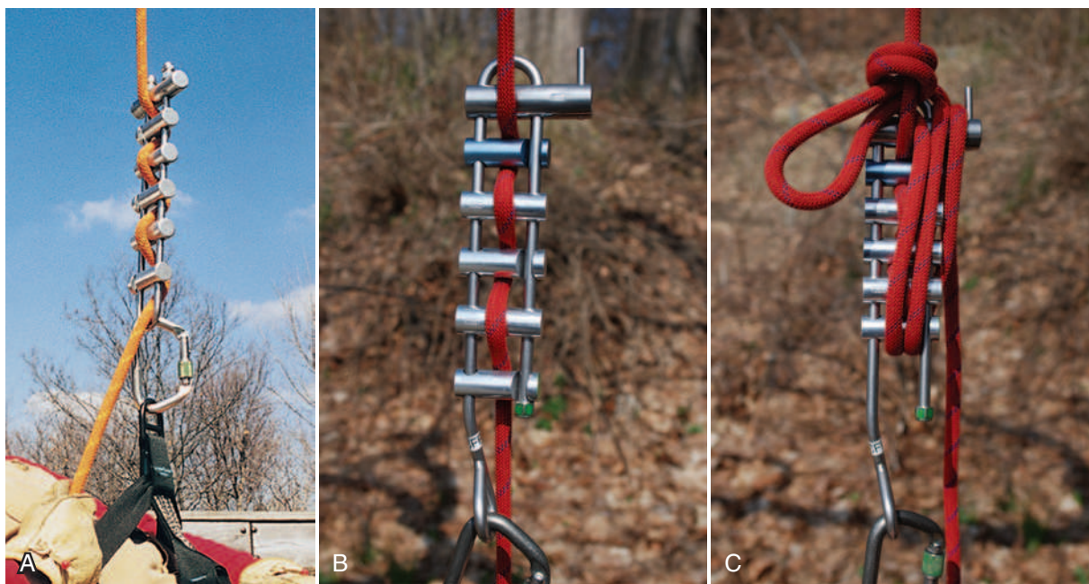
FIGURE 55-23 A, RSI Rigging Rescue Rack brake bar rack in use. B, SMC National Fire Protection Association brake bar rack with welded eye twisted 90 degrees; configured for use. The top bar has been modified to allow for a secure tie-off. C, Brake bar rack tied off. When the bars are pulled tightly together, excessive friction prevents movement on the rope. (Courtesy DC Copper.)
