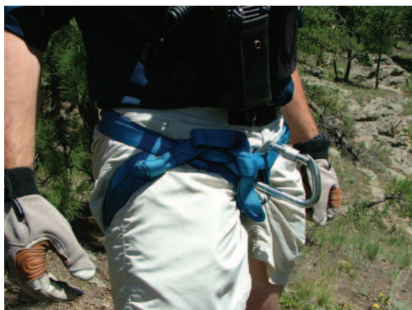
FIGURE 56-14 “Swiss” seat harness; a tied harness using webbing. (Courtesy Loui H. McCurley.)
