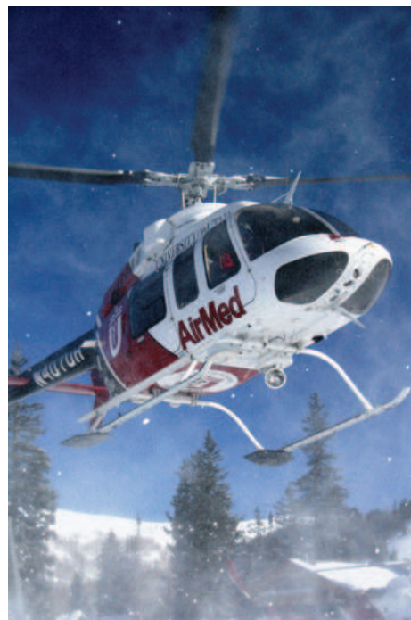
FIGURE 58-13 The Bell 407 appears similar to the Bell 206 (see Figure 58-2 ), but its manufacturer-recommended service ceiling (i.e., maximum operational altitude) is nearly twice as high. (Eric Swenson, University of Utah AirMed.)
