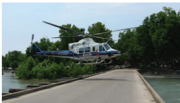
FIGURE 58-19 Bell 412 EMS helicopter landing on a low bridge in the Texas hill country. Although small, this landing zone offers good approach and departure paths with minimal obstacles. Traffic over the bridge should be stopped at a minimum of 30.5 m (100 feet), and preferably more, away from the landing zone during approach, landing, and takeoff. (Courtesy San Antonio AirLife.)
