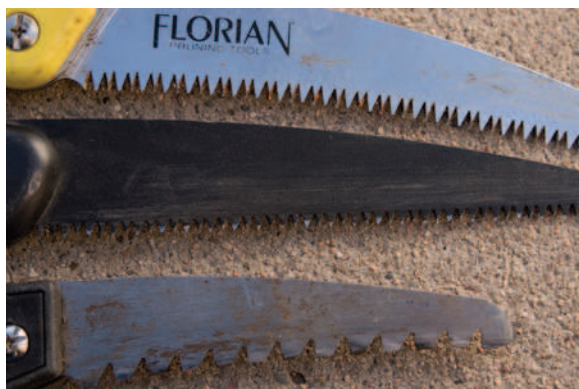
FIGURE 59-48 Pick a saw that cuts in both directions and has aggressive teeth.
