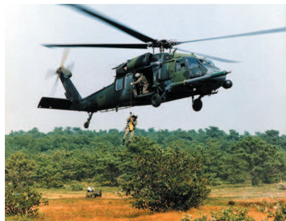
FIGURE 58-3 An MH-60G Pave Hawk hoists a pararescuer during a search and rescue exercise. The S-60 variant includes modifications such as forward-looking infrared, night vision-compatible cockpit lighting, terrain and navigation radar, auxiliary fuel tanks, and hoist. The aircraft can be refueled while in flight. (Courtesy of U.S. Air Force.)
