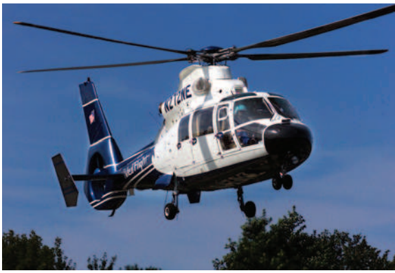
FIGURE 58-22 The AS-365 (N2 variant) is one of the larger, faster twin-engine helicopters used in air medical transport. (Courtesy Boston MedFlight.)
