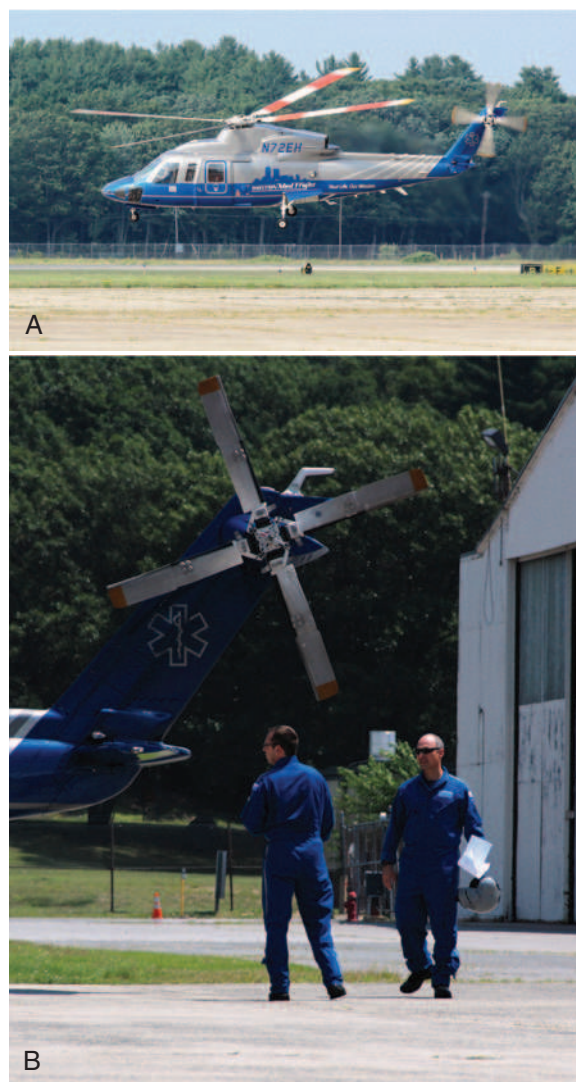
FIGURE 58-26 A, The Sikorsky S-76 is one of the larger twin-engine helicopters used in U.S. air medical transport. B, Among the S-76's advantages that may be less obvious is the additional safety margin provided by the high positioning of the tail rotor (see also Figure 58-16C depicting tail rotor height on AgustaWestland 139). It should be noted that the crew would not be in the depicted positions if the rotor were turning. (Courtesy Boston MedFlight.)
