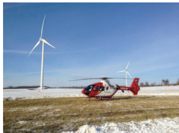
FIGURE 58-33 Landing zone setup must take careful account of high nearby obstructions. (Courtesy Michael Abernethy and Ryan Wubbens, University of Wisconsin Med Flight.)
