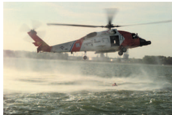
FIGURE 58-11 U.S. Coast Guard HH-60J Jayhawk helicopter (like the Black Hawk, an S-70 variant) in low hover over water, preparing to lower hoist cable to the rescue swimmer. Note the extensive spray under the aircraft. (Courtesy U.S. Coast Guard.)
