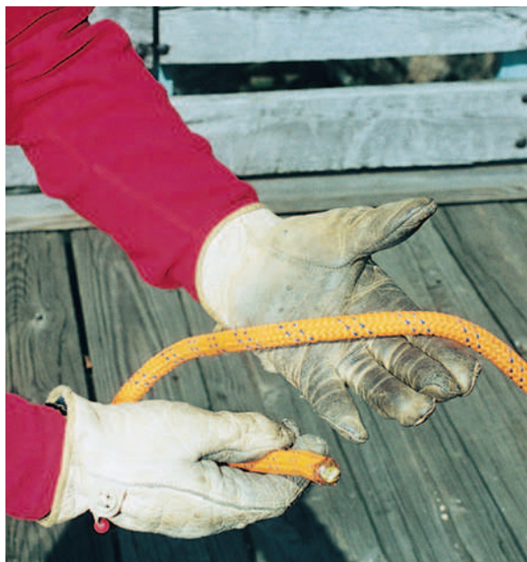
FIGURE 55-17 Example of 13-mm (0.5-inch), nylon, static, kernmantle rope of the type commonly used in rescue. Rescue rope should be checked over its entire length for damage before use. (Courtesy DC Copper.)
