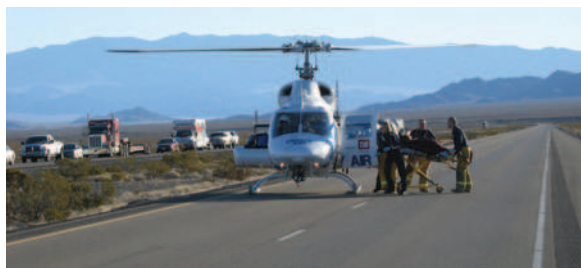
FIGURE 58-20 Emergency medical services Bell 222 helicopter landing on a freeway near the Nevada Test Site, 96.6 km (60 miles) north of Las Vegas. Note that traffic in both directions of the freeway has been stopped. (Courtesy Nevada Test Site Fire-Rescue.)
