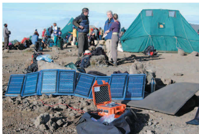
FIGURE 109-54 These rigid solar arrays provide more than 50 W of power under equatorial sun on Mt Kilimanjaro. They weigh less than 4.5 kg (10 lb). This power is controlled by an electronic voltage regulator using a lead-acid battery storage system, housed in the orange, waterproof case in the foreground (6.3 kg [14 lb]). (Courtesy N. Stuart Harris.)
