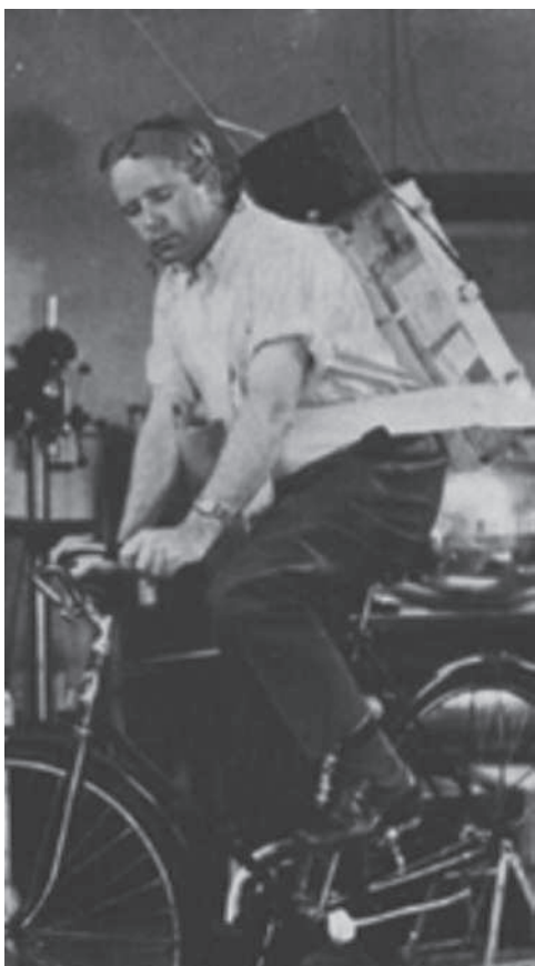
FIGURE 104-3 Tele-electrocardiography. Norman Holter demonstrating his radio-electrocardiograph while riding a bicycle in 1947, the first documented use of portable ECG monitoring. The device weighed 38 kg (84 lb). (From Ioannou K, Ignaszewski M, MacDonald I: Ambulatory electrocardiography: The contribution of Norman Jefferis Holter , BC Med J 56(2):86-89, 2014.)
