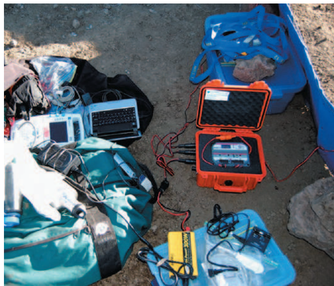
FIGURE 109-55 Electronic devices employed in the field on a solar-powered, high-altitude ultrasound research expedition on Mt Kilimanjaro in association with the U.S. Army and Explorers’ Club. Left to right, The ultrasound unit (SonoSite 180), laptop data storage (Dell Inspiron 910), DC-to-AC converter (bright-yellow box in foreground, Go Power! 300-W converter), electronic voltage regulator with lead-acid battery storage (orange box, CT Solar.com) with 54-W solar arrays (at far right, CT Solar.com). Total weight of all electronic and power storage equipment was less than 18 kg (40 lb). (Courtesy N. Stuart Harris.)
