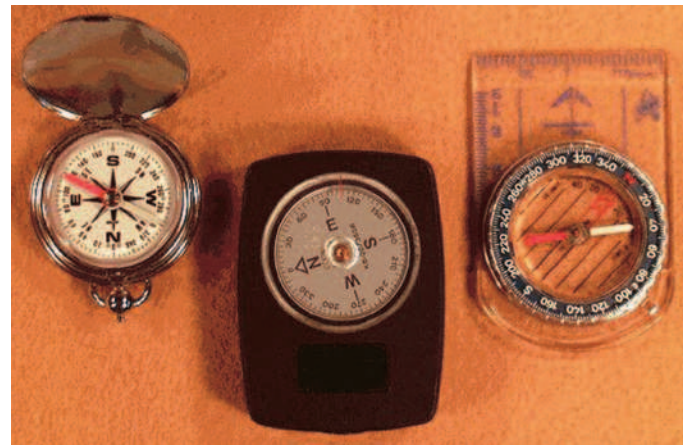
FIGURE 106-9 The three basic compass types. From left to right: Fixed-dial compass, magnetic card compass, and baseplate compass. Note the deviation in indicated north resulting from local magnetic influences.
