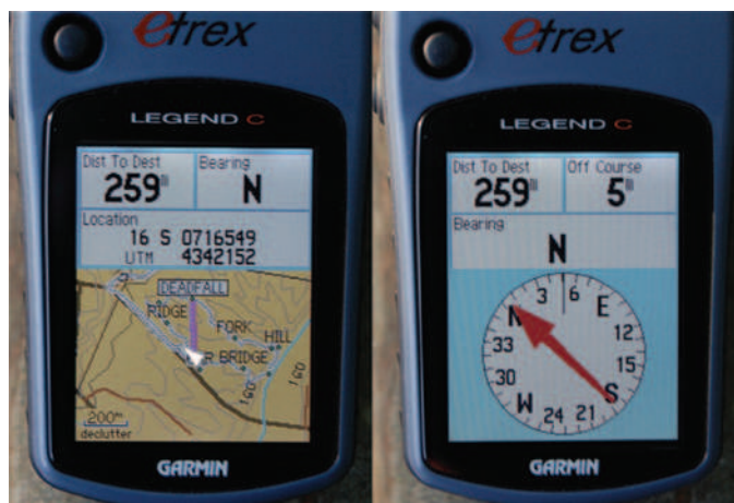
FIGURE 106-3 A typical GPS receiver showing two navigation screens. The screen on the left displays the terrestrial coordinates of the user’s position in the Universal Transverse Mercator format, with a moving map that shows the current position (indicated by the ▲ symbol) and several labeled waypoints. The tracks made by the user when walking the route are shown as a continuous line of small dots. A pink line shows the bearing line from the user’s starting location to a selected waypoint (i.e., “DEADFALL”). The data fields display the distance to the waypoint in meters and the true bearing to the waypoint. North is at the top of the screen. The screen on the right shows the bearing and distance to the selected waypoint and a graphic representation of the direction of travel to the waypoint. The data field in the upper right corner displays the distance in meters that the hiker is off of the line between the original position and the waypoint. If the user walks a course that minimizes the deviation from this line, the waypoint will be gained. If the user is forced to detour by terrain features, he or she can return to the line to get back on course. Note the scale indicators (i.e., meter bar at the bottom left of the screen and meter ring around the current position of the hiker).
