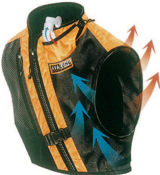
FIGURE 102-4 The AvaLung is a lightweight vest designed to improve avalanche survival. Victims are able to draw air from even a dense snowpack through the front using an air-exchange mouthpiece. A one-way valve permits exhalation of carbon dioxide, which is expelled through the back of the vest. (Courtesy Black Diamond, Ltd.)
