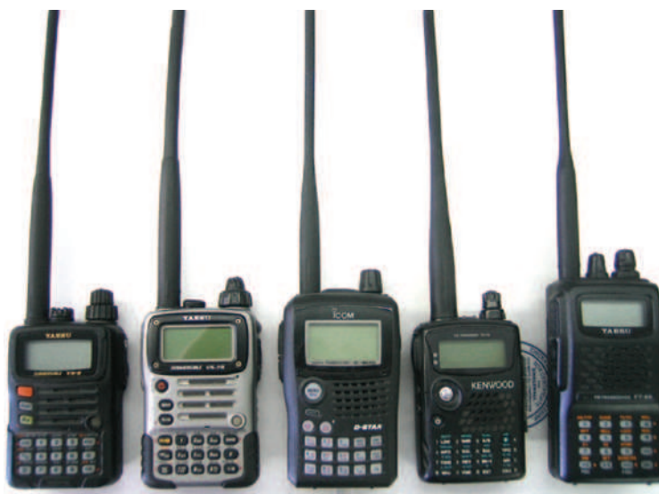
FIGURE 105-2 A selection of small, handheld handy talkies (HTs). These radios communicate on the 2-m (144-MHz) and 70-cm (420-MHz) amateur radio service bands. HTs are more capable and rugged than FRS, GMRS, and FHSS radios, but their use requires FCC licensure through a process that includes testing on radio theory, equipment, procedures, and regulations. The radios pictured here use rechargeable lithium ion batteries.
