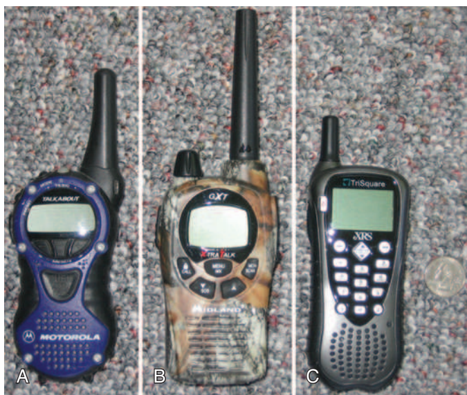
FIGURE 105-1 Several inexpensive handheld radios for short-distance communication. A and B , Hybrid Family Radio Service (FRS)/General Mobile Radio Service (GMRS) transceivers. C , 900-MHz (33-cm band) frequency-hopping spread spectrum (FHSS) radio. A common coin is pictured to provide scale. All three radios can be powered by rechargeable battery packs or disposable AA batteries. The FRS/GMRS radios require a license from the U.S. Federal Communications Commission (FCC) to transmit on the higher-wattage channels unique to the General Mobile Radio Service.
