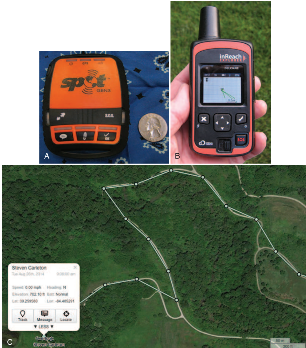
FIGURE 105-4 A, Satellite messenger with a common coin provided for scale. Note that the user interface consists of only four buttons and four indicator light-emitting diodes. The “HELP” and “9-1-1” buttons are recessed to prevent accidental activation. During routine use, the unit is turned on and given several minutes to establish a GPS fix, and the “OK” button is pressed to send the current coordinates and a preplanned check-in message to the cell phones or e-mail addresses of individuals designated by the user. Battery power is sufficient for hundreds of such check-in messages. B, Satellite communicator that permits simple GPS navigation as well as the functions described in A. This device also allows two-way satellite text communication using a virtual keyboard. C, Demonstration of the GPS tracking function supported by the device shown in B. GPS coordinates are sent via satellite at intervals determined by the user to a Web page that plots the user’s location on a map or satellite image for each check-in time. Messages from the user can be appended to each plotted point to allow emergency contacts, family members, expedition support personnel, or media to follow the progress of a wilderness excursion.
