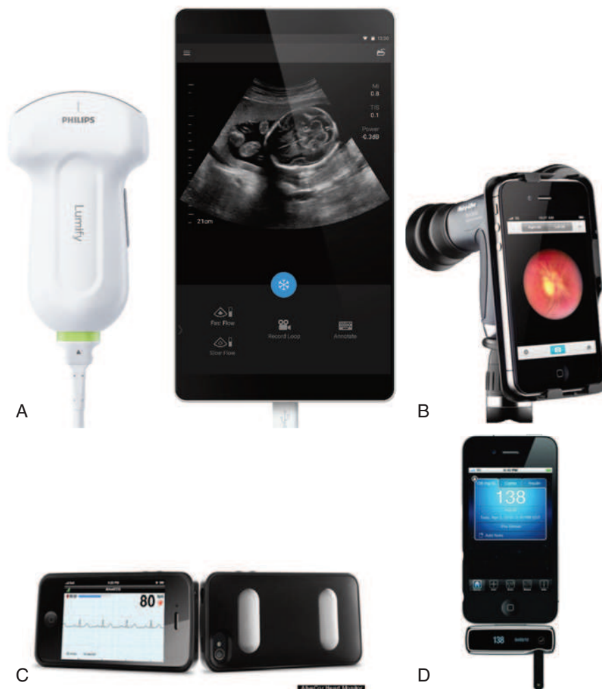
FIGURE 104-4 Smartphone telemedicine. Miniaturization of biologic sensors and medical devices allows remote monitoring or diagnostics for use in the field. A , The Philips Lumify, a portable ultrasound designed for a mobile smart device. B , WelchAllyn iExamine, an iPhone-compatible funduscope. C , AliveCor Heart Monitor, a smartphone-based ECG machine. D , Sanofi iBGStar, an iPhone-based glucometer. (A courtesy Philips Ultrasound Inc, Andover, MA; B courtesy WelchAllyn, Skaneateles Falls, NY; C courtesy AliveCor, San Francisco; D courtesy Sanofi, Bridgewater, NJ.)
