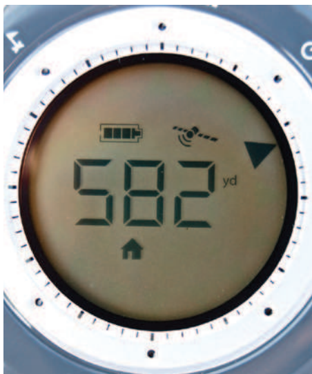
FIGURE 106-2 A simple, single-function, Global Positioning System (GPS) receiver. The screen displays the distance to a known waypoint (designated by the “house” symbol) and has an arrow on the rim that points in the direction of the waypoint. As the user hikes in the direction indicated by the arrow, the distance counts down and, in the absence of obstructions to travel, the waypoint is gained.
