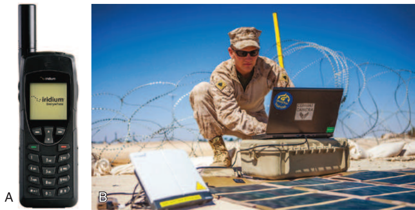
FIGURE 105-3 A, Typical satellite telephone. The antenna on most satellite phones folds for travel and must be extended and held vertically to optimize performance. Satellite phones are becoming smaller as technology evolves. B, Representative Broadband Global Area Network (BGAN) terminal. This device is plugged into the USB port of a laptop and oriented so that the integral antenna faces the GEO satellite for the region in question to provide satellite Internet service. A BGAN terminal allows standard voice communication and data transfer for text or e-mail and has the capacity to stream larger volumes of data at transfer rates that allow smooth, real-time video to be transmitted and received. Applications for telemedicine are promising. (A Iridium 9555 Satellite Phone courtesy Chroma Communications, Inc; https://satellitecommunications.ca/product/iridium-9555-satellite-phone .)
