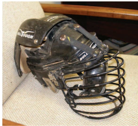
FIGURE 37-16 Bull-riding helmet damaged after impact with bull's hoof. (Courtesy Mark Brandenburg, MD.)
