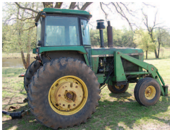
FIGURE 37-8 Tractor with rollover protection structure (ROPS). (Courtesy Mark Brandenburg, MD.)
