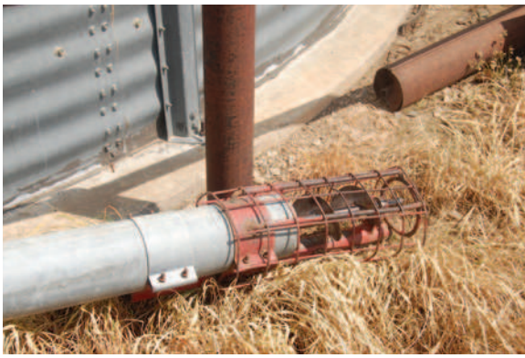
FIGURE 37-9 Auger with shielding. (Courtesy Mark Brandenburg, MD.)
