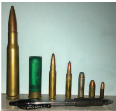
FIGURE 27-23 Comparison of different common ammunition sizes. Left to right: .50 caliber BMG (Browning Machine Gun), 12-gauge shell (shotgun), .308 (rifle), .223/ 5.56 mm (used in AR-15, M-16 rifles), .357 (pistol), 9 mm Parabellum hollow point (pistol), .22 LR hollow point, and pen for size comparison. (Courtesy N. Stuart Harris, MD.)
