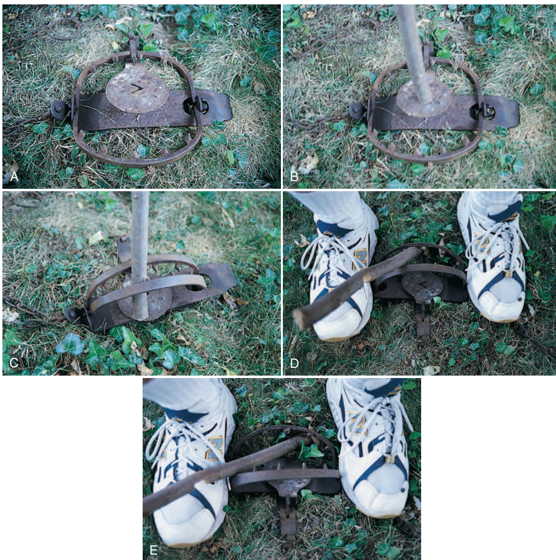
FIGURE 26-16 A, A leghold trap set. B and C, A leghold trap sprung. D and E, To release a trap that has been sprung, stand on each end of the trap and compress the spring.
