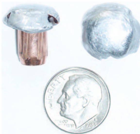
FIGURE 26-13 The .30-caliber Nosler 180-g AccuBond Polymer Tip bullet fired into calibrated 10% ordnance gelatin is typical of the .30-caliber hunting bullets used for .30-06, .308, .300 Win Mag, and other cartridges. This photo shows this bullet fired from a .308 rifle with a 45.8 cm- (18-inch) long barrel. Muzzle velocity was 762 m/sec (2499 feet/sec). Penetration depth exceeded 50.8 cm (20 inches). Temporary cavity maximum width was 11.4 cm (4.7 inches) at a depth between 7.1 cm (2.8 inches) and 22.1 cm (8.7 inches). Diameter of the recovered bullet at the front surface was 1.4 cm (0.6 inches). Weight of the recovered bullet was 149.5 g (5.3 oz); 17% of the bullet turned into fragments. Terminal performance of this type is suitable for all medium to heavy game encountered in the lower 48 U.S. states, including moose, elk, black bear, pigs, and deer. Ten-cent coin (dime) is shown for comparison. (Courtesy Gary K. Roberts, DDS.)
