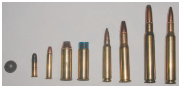
FIGURE 26-11 Examples of hunting bullets. Left to right, .50-caliber black powder lead bullet, .22-caliber long rifle lead bullet, .22-magnum caliber copper jacketed bullet, .44-magnum semijacketed hollow-point bullet, .44-magnum shotshell, .223-caliber (5.56-mm) full metal jacket bullet, .30/30-caliber soft point flat nose bullet, .30-06-caliber round nose soft point bullet, and .270-caliber pointed soft nose bullet.
