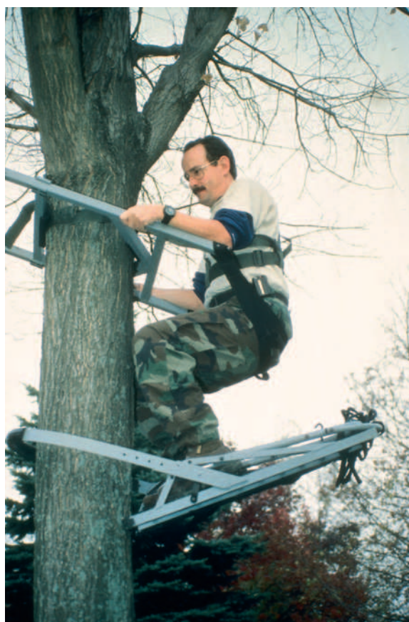
FIGURE 26-2 A commercially produced tree stand can be used to climb the tree and obviates the need for a ladder or steps, which are the cause of many falls.
