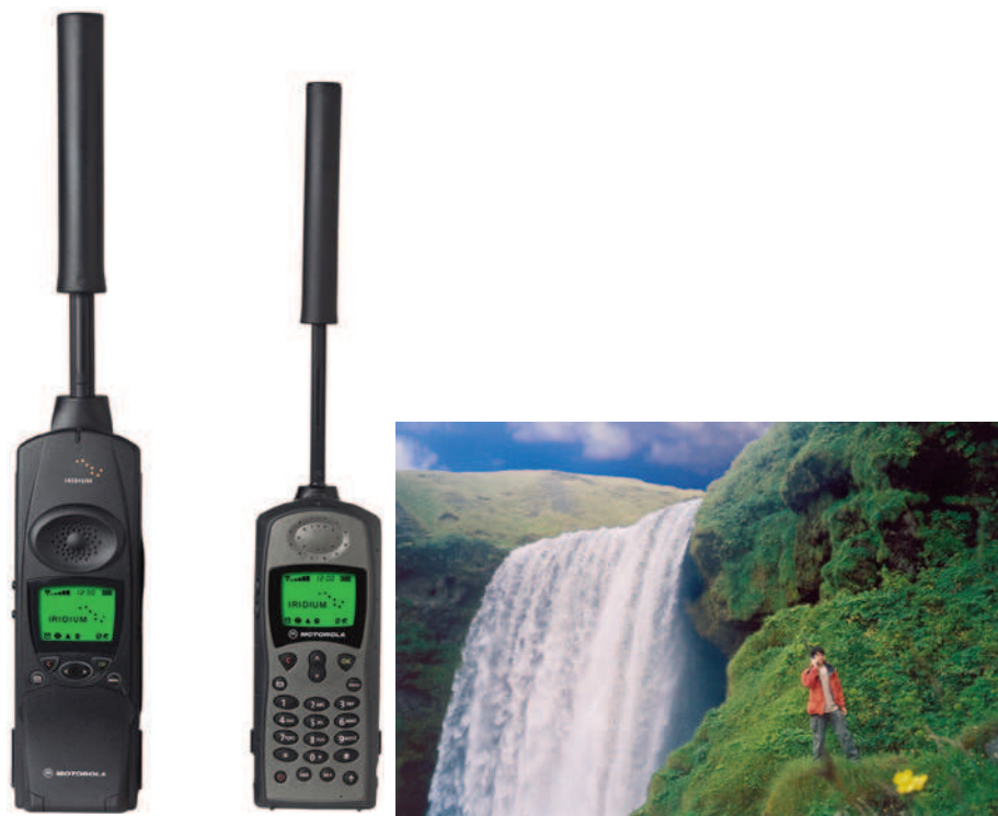
FIGURE 29-3 Compact satellite telephones.
