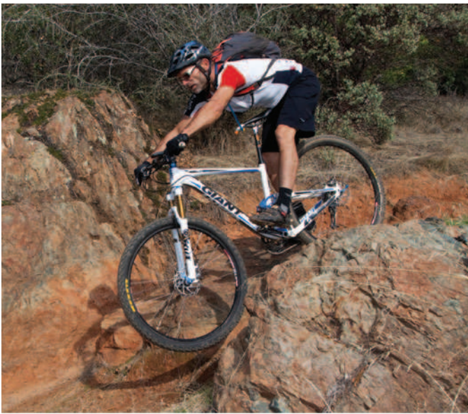
FIGURE 99-5 Modern mountain bicycles are highly specialized pieces of equipment. This bike has front and rear suspensions, disk brakes, and clipless pedals. Such features are common on today's bikes. (Courtesy Dr. Steven J. Wolf.)
