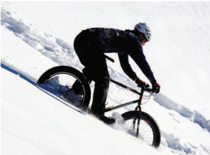
FIGURE 99-6 Fat bikes are increasingly popular versions of mountain bikes. Fat bikes have massive low-pressure tires that allow for riding in unconventional cycling environments, such as through snow and sand. (Courtesy Anthony DeLorenzo.)
