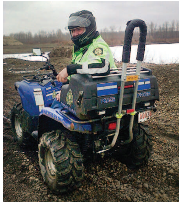
FIGURE 99-21 Crush guard. This safety device is designed to prevent the driver from being crushed by the heavy vehicle in the event of a rollover accident. Its use is not widespread, and its efficacy has yet to be determined. (Courtesy Quadbar Safety: quadbarsafety.com .)
