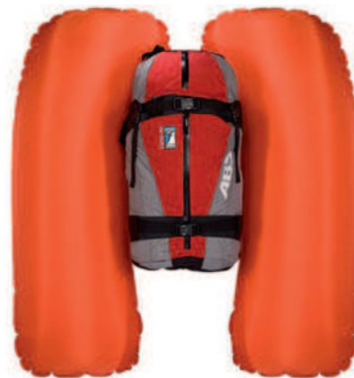
FIGURE 4-19 The German 170-L (5.6-foot 3 ) dual-airbag system (ABS). This device utilizes two wing-like 85-L (3-foot 3 ) balloons inflated by pulling a T-shaped ignition handle, thereby rapidly releasing nitrogen from a canister that draws air into the balloons by a Venturi effect. Although this configuration favors a final prone position close to the surface of the debris, possibly compromising the airway, the manufacturers suggest that the bilateral and posterior position of the balloons affords horizontal stability in the laminar flow of the avalanche.
