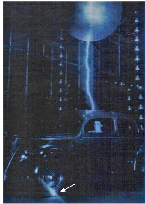
FIGURE 5-8 Simulated lightning in a high-voltage laboratory travels across the external metal body of the car, escaping through the axle, hubcaps, or other metal closer to ground (arrow). The Faraday cage effect of the metal body of the car protects the person from injury but does not protect the tires or wiring system of the vehicle.
