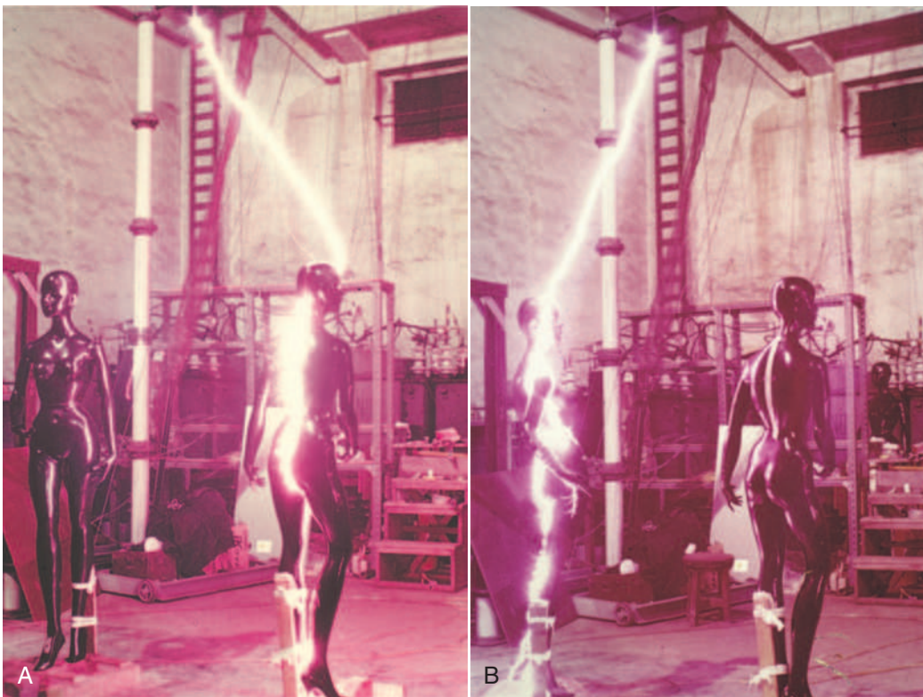
FIGURE 5-45 Simulated lightning strike applied on one dummy coated with metal and the other without. Discharges ran from an electrode equidistant from both and hit each dummy an equal amount of times, showing that metal does not attract lightning, including anything a person wears. (Copyright Nobu Kitagawa; courtesy Mary Ann Cooper.)
