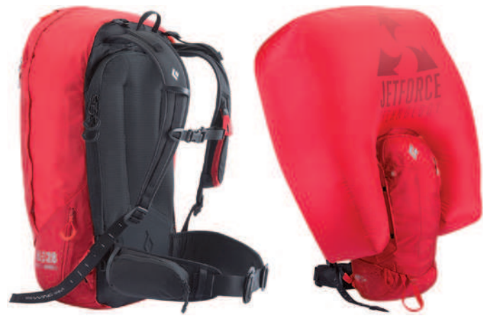
FIGURE 4-21 The JetForce Avalanche Airbag Pack (Black Diamond Equipment) uses a battery-powered fan instead of a compressed gas cylinder. The fan inflates a 200-L (6.9-foot 3 ) airbag in 4 seconds, then automatically deflates the bag after 3 minutes. This system can be deployed, repacked, and ready for use without having to refill a compressed gas cylinder.
