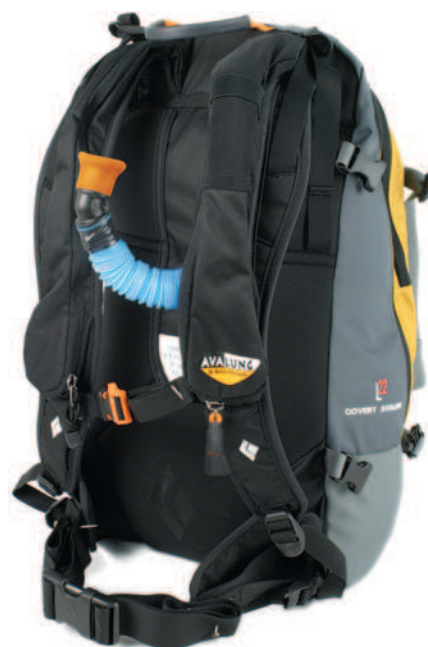
FIGURE 4-24 The AvaLung backpack. A stowable mouthpiece is located in the shoulder strap along with the inspiratory and expiratory valve housing. Inspiratory air enters through a one-way valve in the valve housing located in the shoulder strap and flows through respiratory tubing and the mouthpiece into the lungs. Expiratory air flows through the mouthpiece into the shoulder strap and through a second one-way expiratory valve. Expired air then travels through the respiratory tubing and through the pack to the lower back on the opposite side, where expiratory air is expelled. (Courtesy Black Diamond Equipment, Salt Lake City, Utah.)
