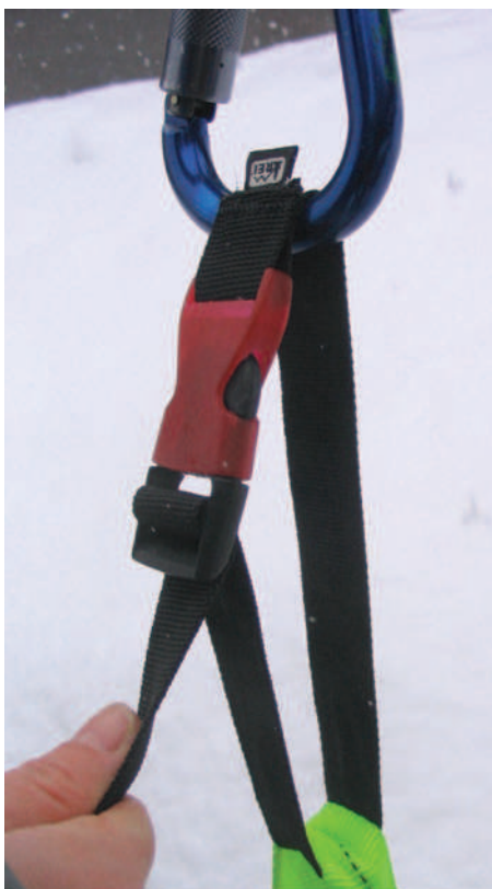
FIGURE 46-63 Fastex-type or cam-lock utility strap makes a very efficient traction device and can be adapted for most systems.
