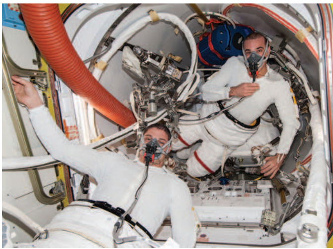
FIGURE 126-2 Astronauts Rick Mastracchio (right) and Mike Hopkins in preparation for a spacewalk in the ISS airlock, breathing 100% oxygen while donning their spacesuits as part of a protocol to reduce the risk of decompression sickness. Note the white cooling and ventilation undergarments that crews wear inside their spacesuits to regulate body temperature.
