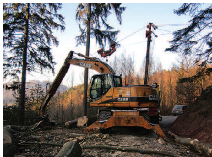
FIGURE 124-11 High-lead cable logging system with loader in the foreground, tower and carriage in background. (Courtesy Donald L. Grebner, Mississippi State University.)
