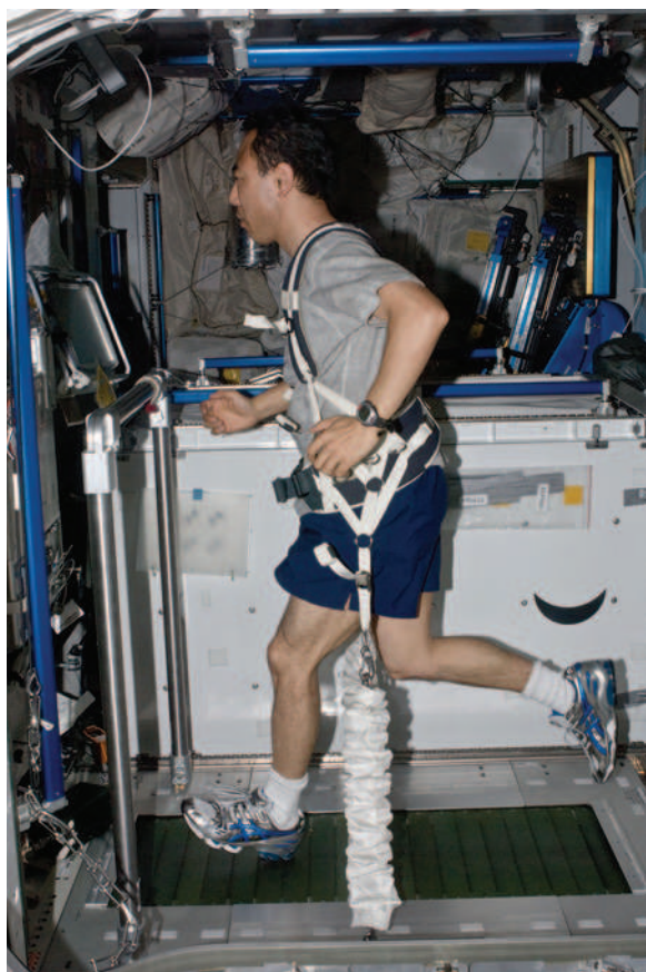
FIGURE 126-8 Astronaut Satoshi Furukawa using the T2, a vibration-isolated treadmill used extensively for exercise aboard the ISS. Note the white loading harness and bungees that pull the astronaut onto the treadmill with a force equivalent to up to 80% of the astronaut's body weight.
