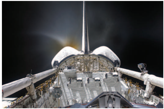
FIGURE 126-4 Emissions visible from the Space Shuttle's orbital maneuvering system during an orbital correction. Once in orbit, nitrogen tetroxide and monomethyl hydrazine are often used to provide thrust to spacecraft.
